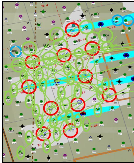
Figure 4.123: Locations of wells showing declining water-cut
