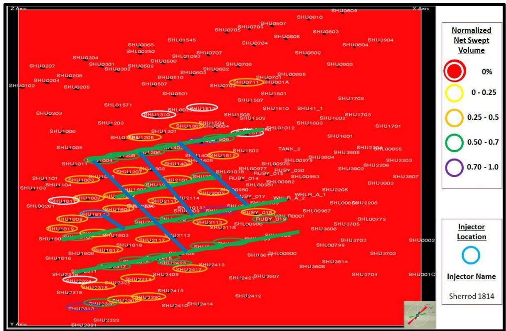
Figure 4.46: 'Sherrod 1814' connectivity with major flow features (green lines) through NW-SE fractures
