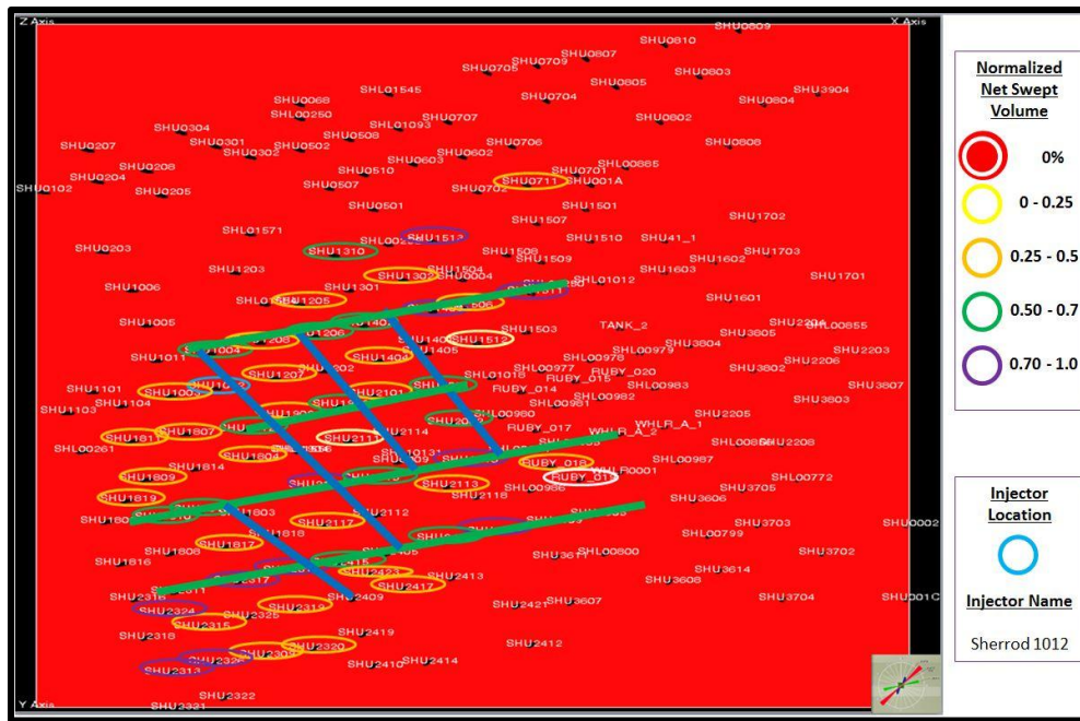
Figure 4.42: 'Sherrod 1012' connectivity with major flow features (green lines) through NW-SE fractures
