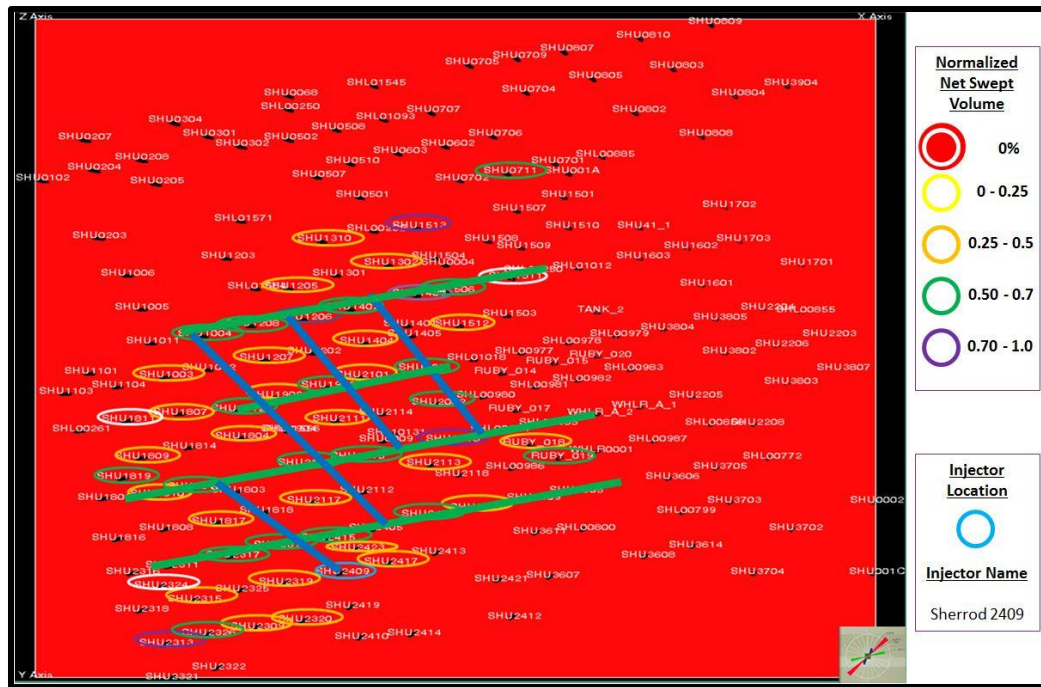
Figure 4.50: ‘Sherrod 2409’ connectivity with major flow features (green lines) through NW-SE fractures
