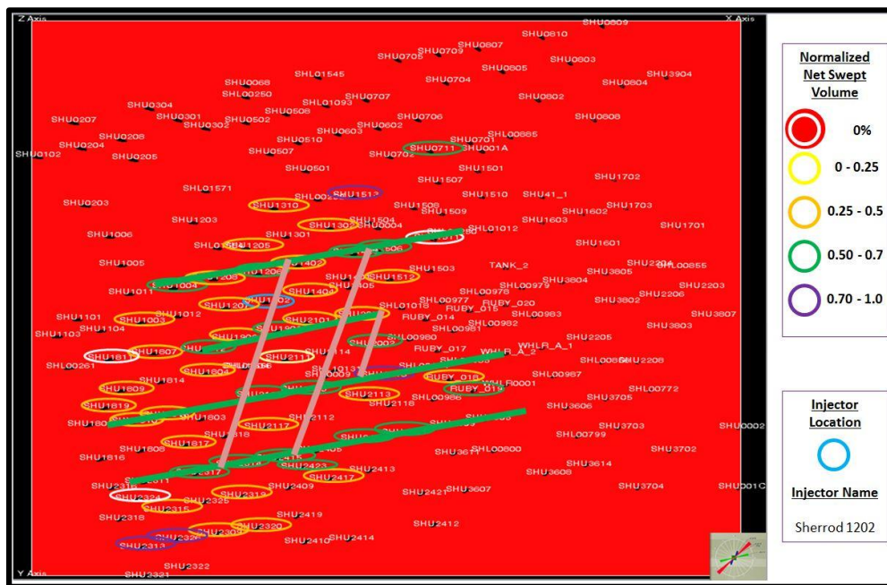
Figure 4.33: 'Sherrod 1202' connectivity with major flow features (green lines) through NE-SW fractures
