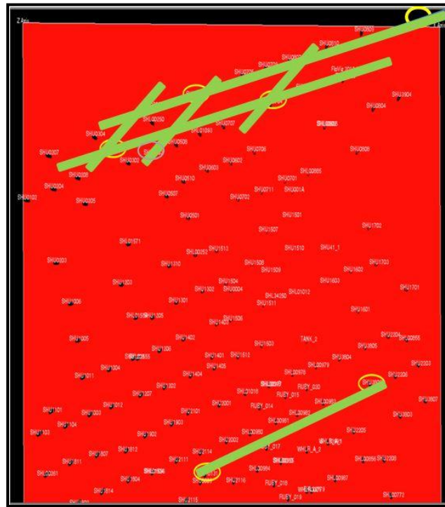
Figure 4.108: Fracture realization from 1973 simultaneous water breakthrough
