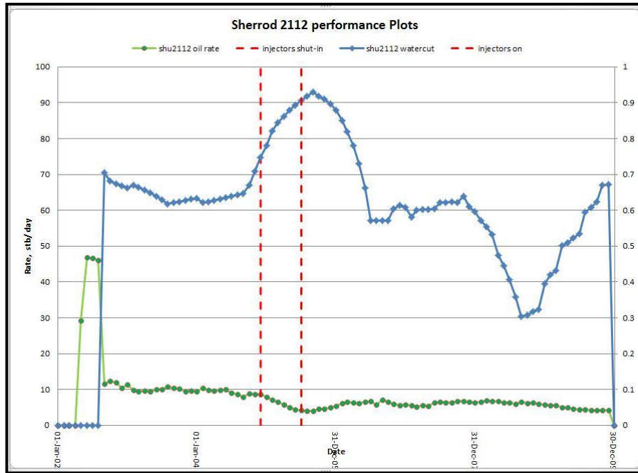
Figure 4.112: Example of water-cut increase during field injection shut-in
