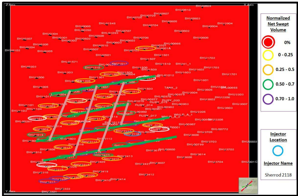
Figure 4.39: 'Sherrod 2118' connectivity with major flow features (green lines) through NE-SW fractures
