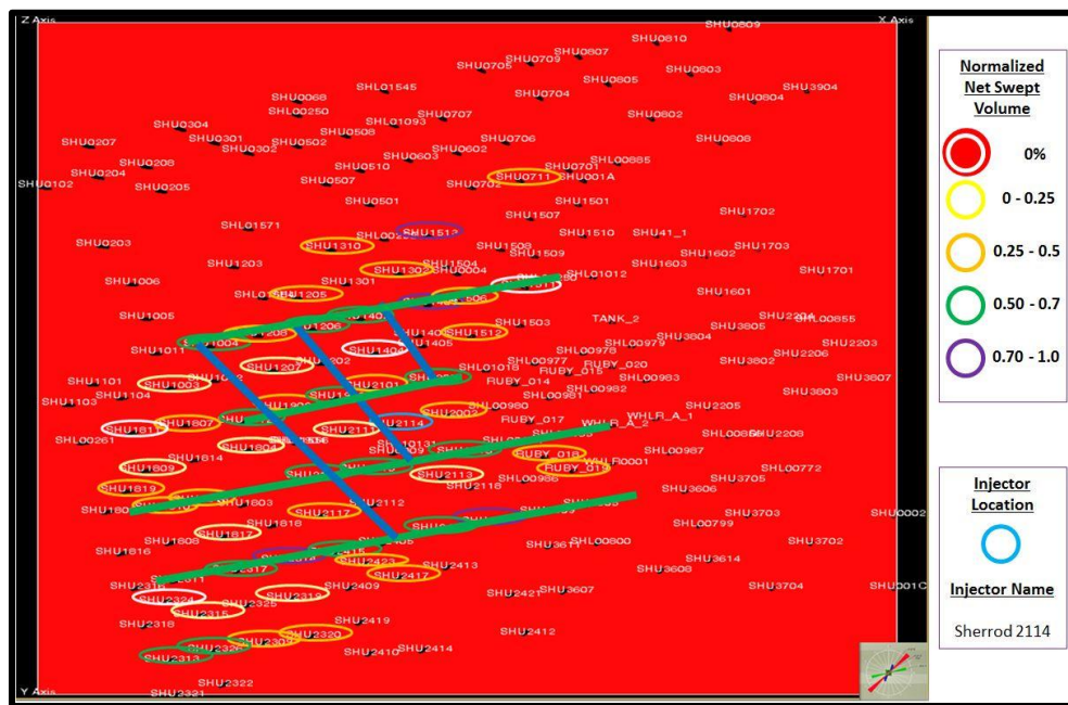
Figure 4.45: 'Sherrod 2114' connectivity with major flow features (green lines) through NW-SE fractures
