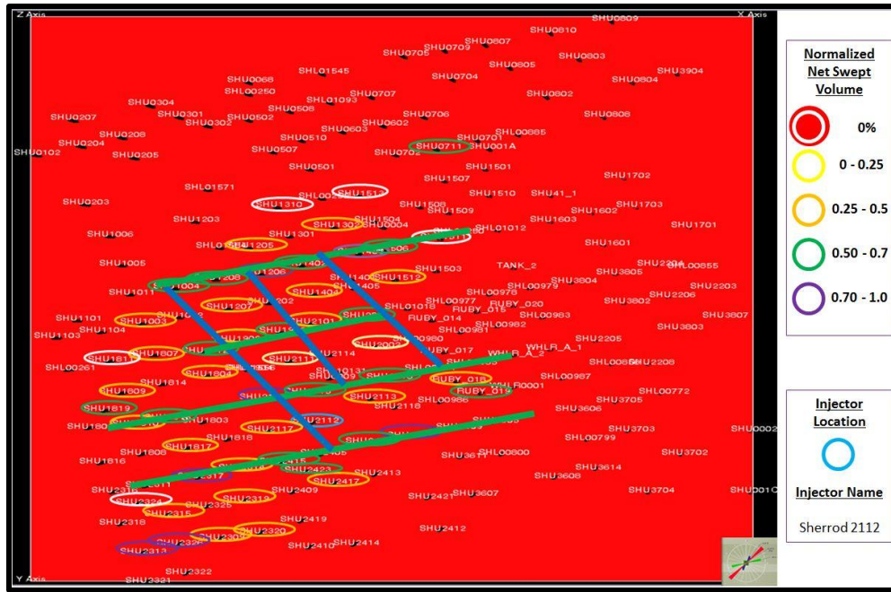
Figure 4.48: 'Sherrod 2112' connectivity with major flow features (green lines) through NW-SE fractures
