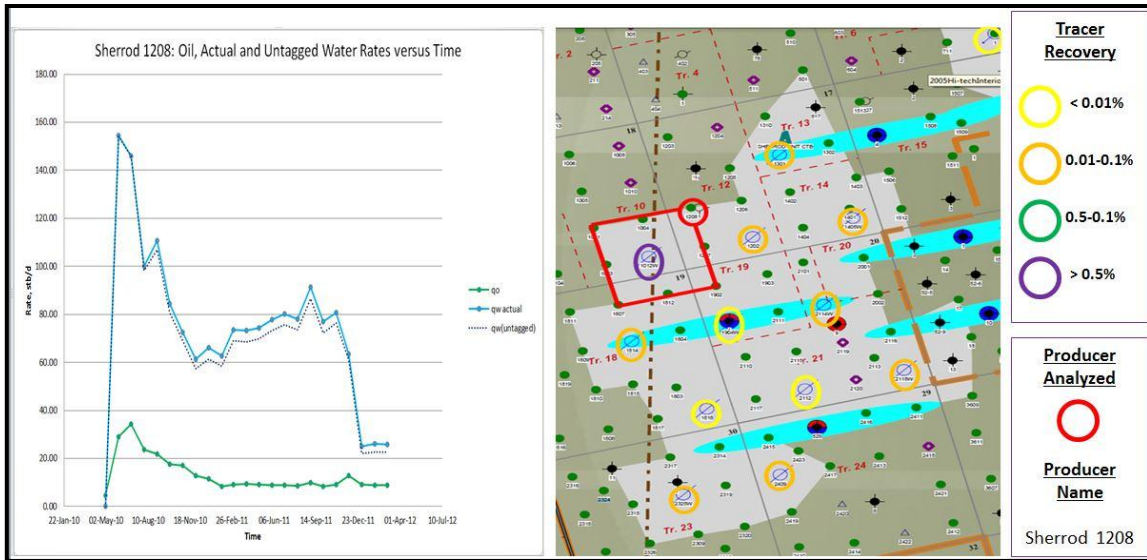
Figure 4.56: Sherrod 1208, contributing injectors, and water rate decomposition.
