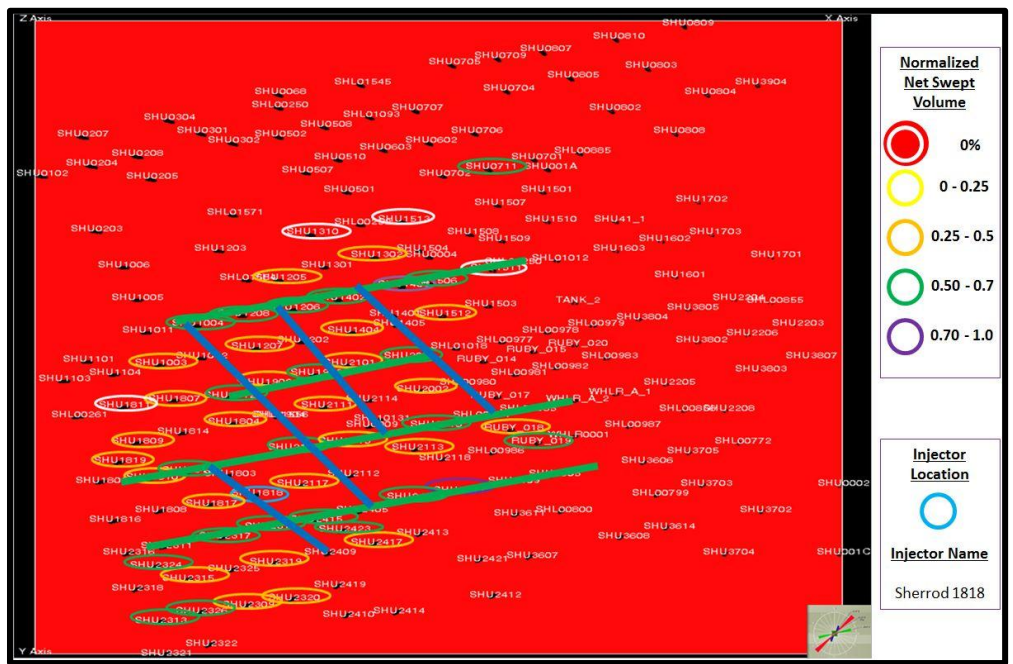
Figure 4.47: 'Sherrod 1818' connectivity with major flow features (green lines) through NW-SE fractures
