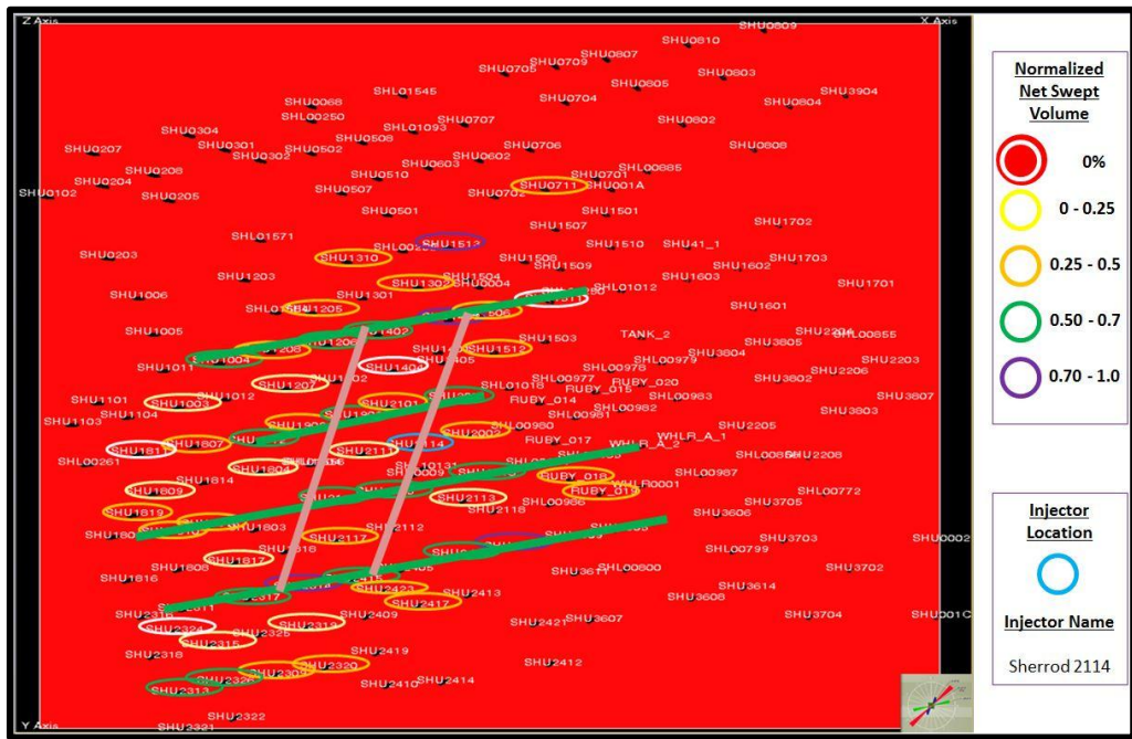
Figure 4.35: 'Sherrod 2114' connectivity with major flow features (green lines) through NE-SW fractures
