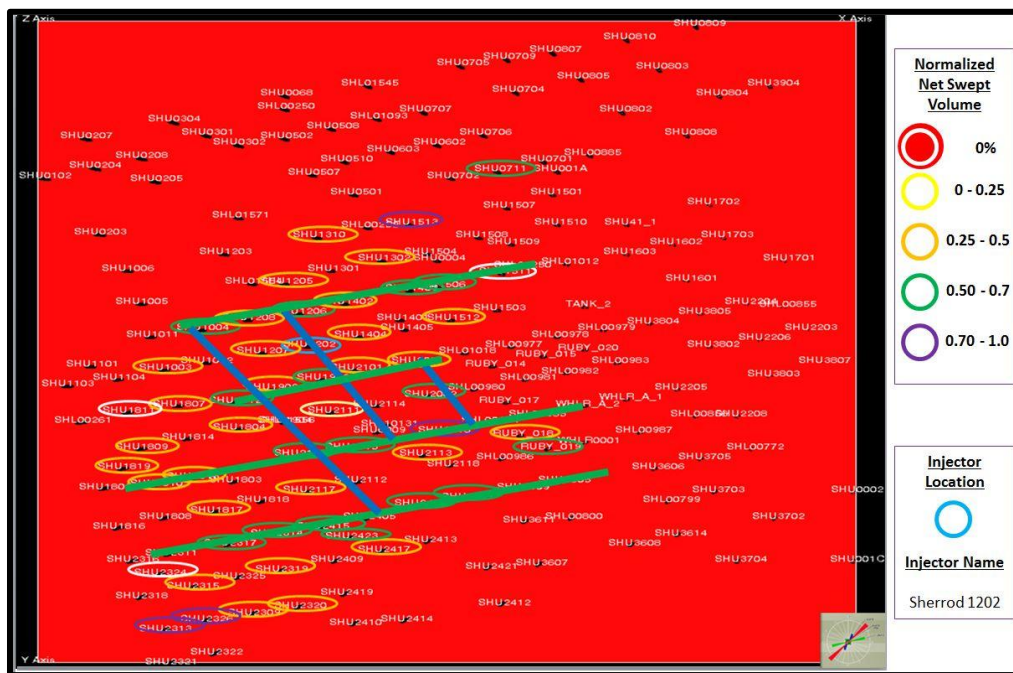
Figure 4.43: 'Sherrod 1202' connectivity with major flow features (green lines) through NW-SE fractures
