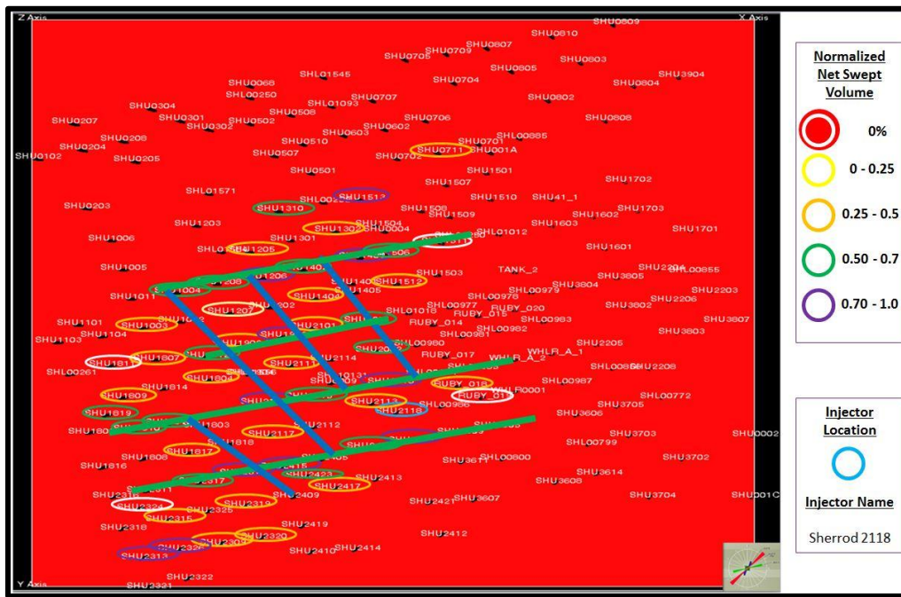
Figure 4.49: 'Sherrod 2118' connectivity with major flow features (green lines) through NW-SE fractures
