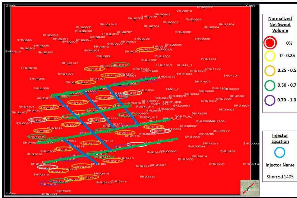
Figure 4.44: 'Sherrod 1405' connectivity with major flow features (green lines) through NW-SE fractures
