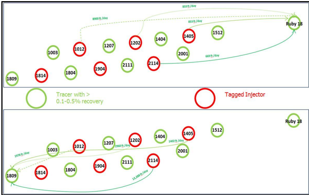
Figure 5.44: The two opposite in direction ultra-high tracer velocities observed from same injectors
