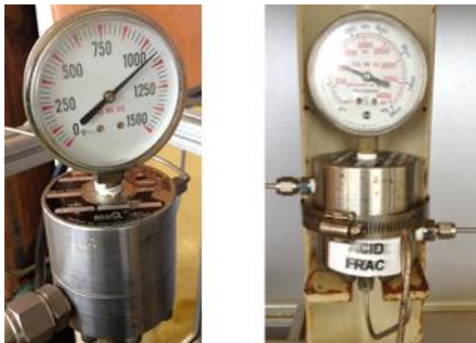
Figure 11: Backpressure regulators used in the acid etching setup
