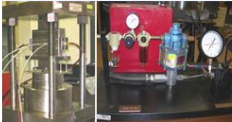
Figure 8: Load frame capable of exerting 10,000-psi closure stress
