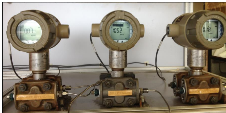
Figure 7: Pressure transducers used in dynamic etching test experiment
