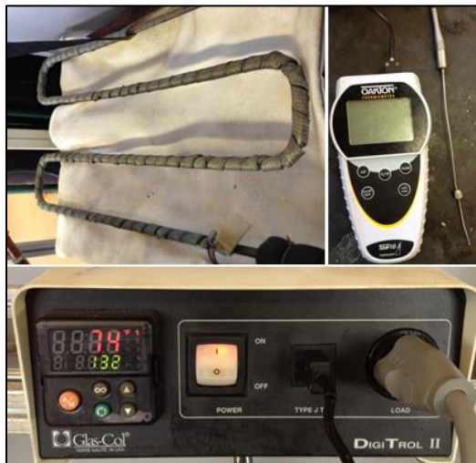
Figure 12: Heating tapes, thermocouple, and temperature control panel
