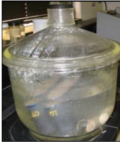
Figure 9: Vacuum pump for saturating cores with tap water
