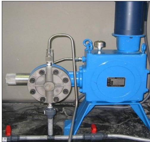
Figure 6: Diaphragm pump capable of pumping 1.4 l/min at max pressure of 2,200 psi
