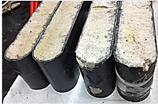
Figure 34: Condition of cores after conductivity test: cores etched with 90% spent (left) acid compared to cores etched with live acid (right)
