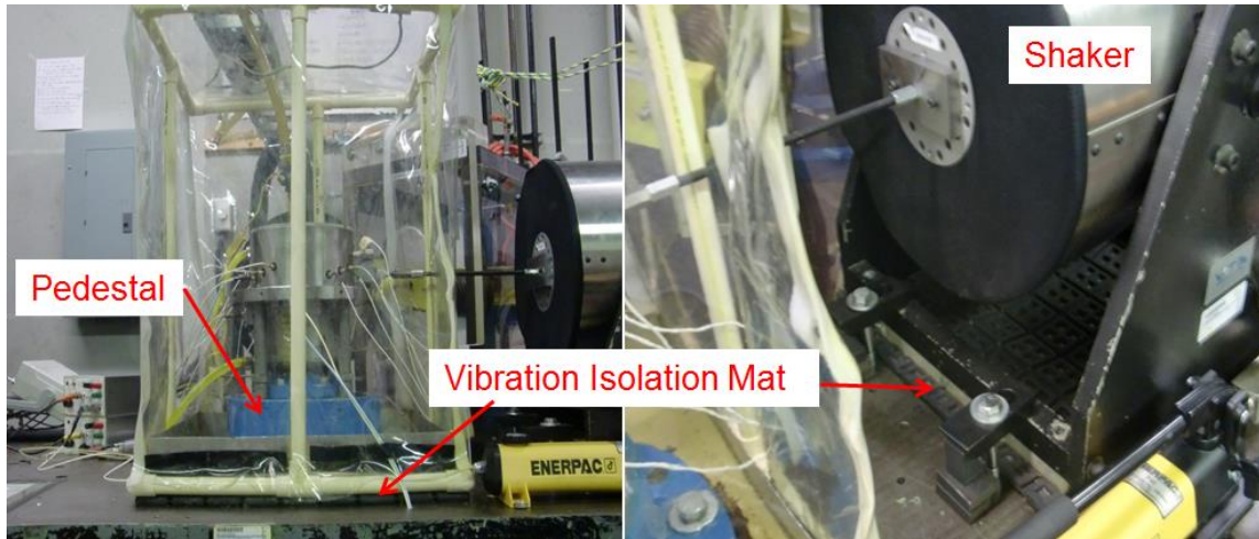
Figure B 2. Side view of SFD test rig and X-Shaker showing the location of the vibration isolation mat
