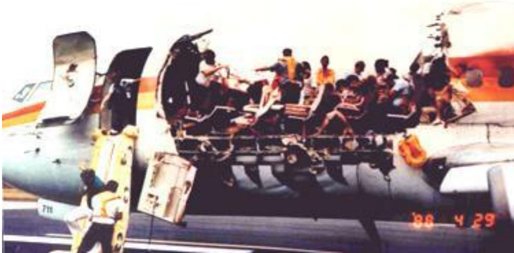
Figure 2. Accident of Aloha airlines aircraft Boeing 737[7]
