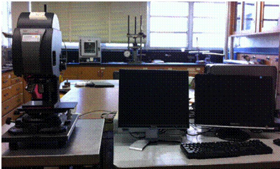
Figure 28. Surface interferometer (ZYGO NEW VIEW 600)
