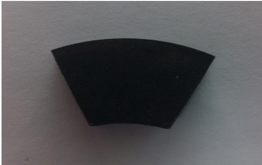
Figure 25. The carbon steel sample for active composite coating for wear protection
