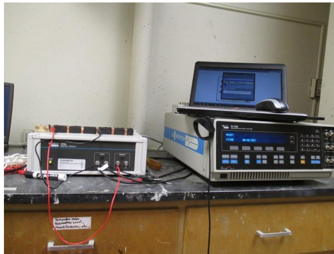
(b) Resistivity measurement set-up: Solartron 1296 & 1260A
