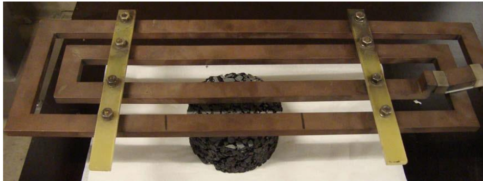
Figure 10. Test set-up for induction heating (Liu et al. 2010b)
