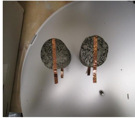
(b) Installing copper tapes as electrodes
