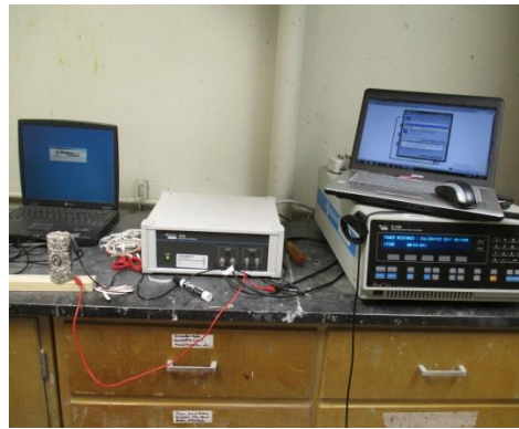
(c) Electrical resistivity measurement devices: Solartron 1260A and 1296.
