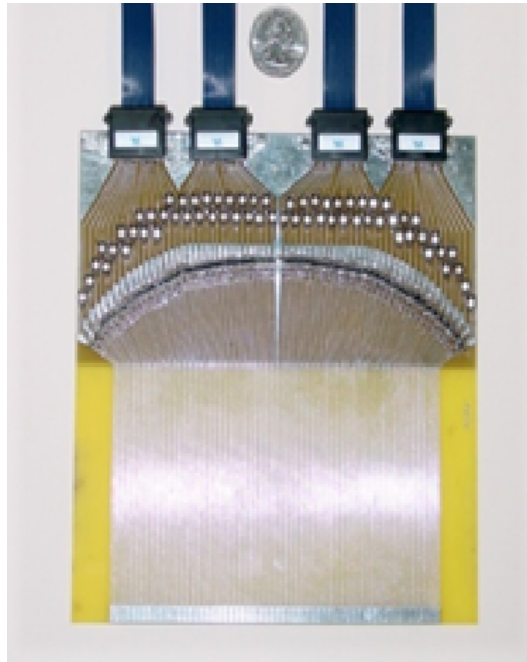
Figure 1.1: The SEA linear array built in Texas A&M University with 64 channels
