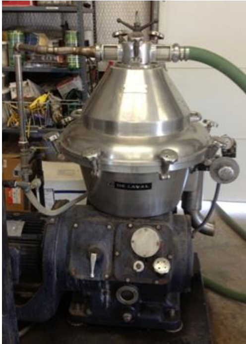
Figure 1. The centrifuge used in Pecos, TX for pilot scale harvesting
