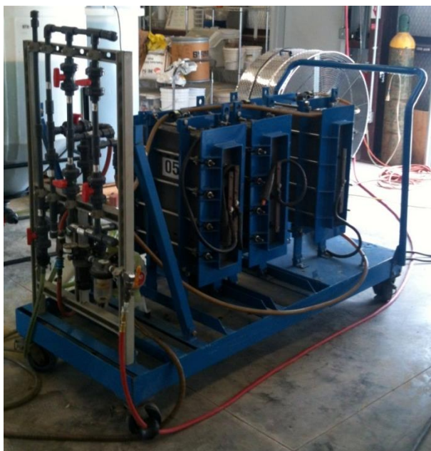
Figure 5. The KASELCO 2.5 gpm reactor test bed configurations. Reactors mounted are 05, 07, and 11.
