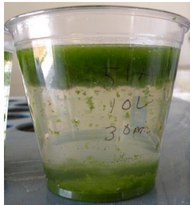
Figure 13. Algae coagulating and floating in tests 4 and 5
