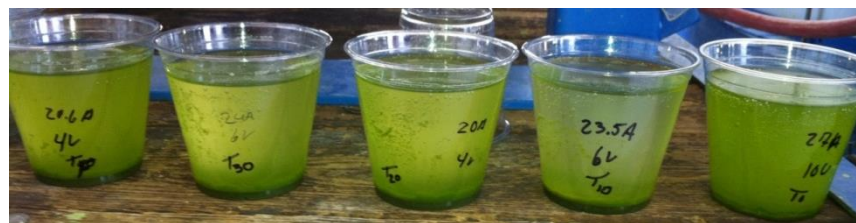
Figure 11. Test 1 partially coagulating algae but did not achieve sufficient removal rates
