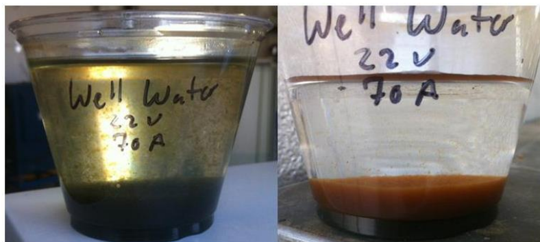
Figure 20. Metal content introduced to well water by electrocoagulation after treatment and stratified layers of metal in well water after 24 hours of settling
