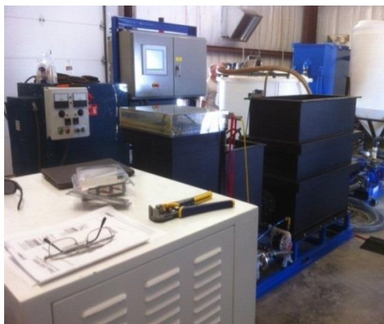
Figure 6. KASELCO's 10 gpm Hi-Flow reactor in the 09 configuration and rectifier system used to harvest 4550 gallons of microalgae
