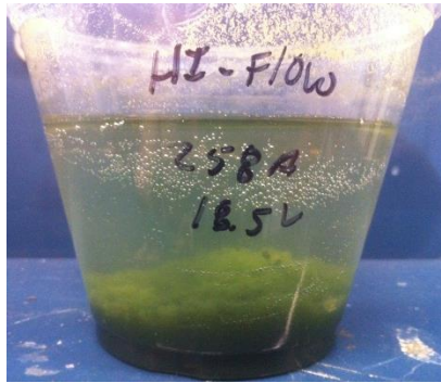
Figure 21. Test 1, 500 gallons, successfully coagulated algae using KASELCO's 10 gpm Hi-Flo reactor
