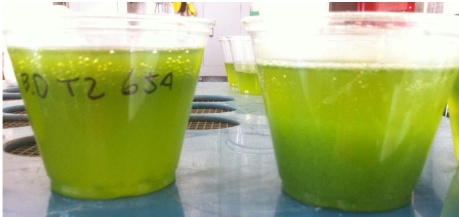
Figure 16. 2012 test using aluminum electrodes failed to remove microalgae from water
