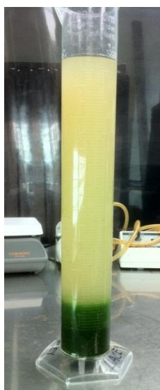
Figure 9. Sedimentation of N. oculata following the addition of PolyDAD polymer
