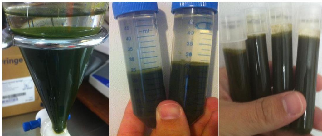
Figure 19. Algal biomass continuing to settle after treatment allowing for more water removal
