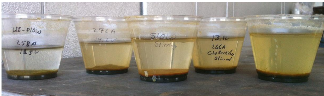
Figure 22. Consistency of removing algae using the Hi-Flo reactor harvesting 4550 gallons
