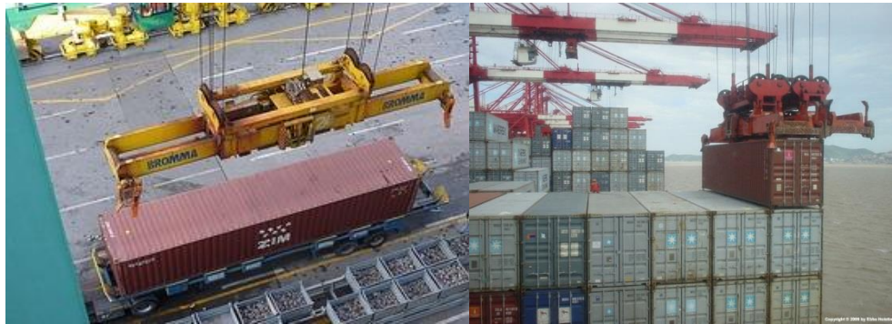
(a) Conventional single-trolley quay crane
