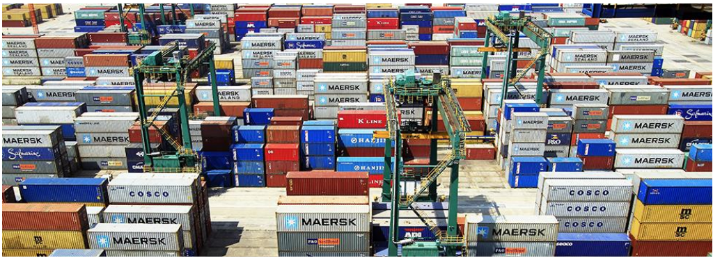
FIGURE 7 RTGs at the storage blocks.
