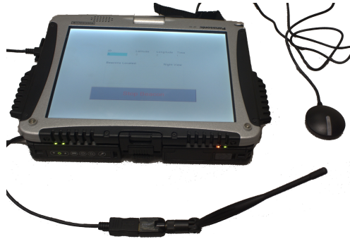
Figure 5.1: Assembly point broadcast hardware with external Wi-Fi antenna and GPS receiver.
