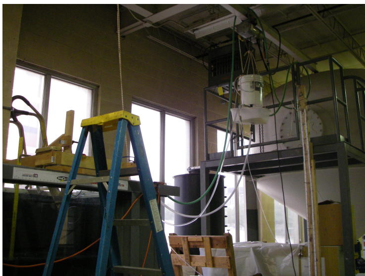
Figure 2.1: Suspended constant head tank at maximum vertical extent and experimental tank
