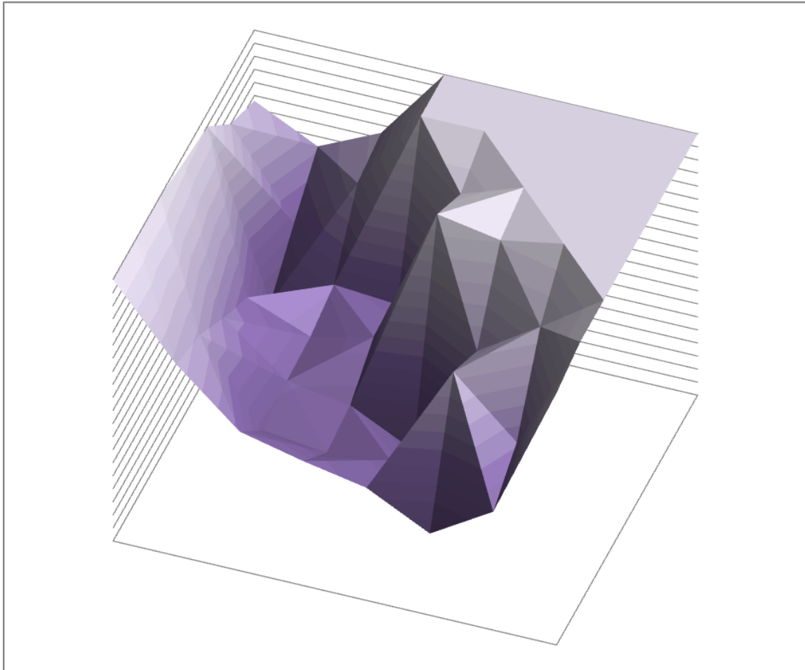
Figure 31. 3D graph of the slow thermalization induced fission probability in the y-axis, the die-away ( \mu s) in the x-axis, and the LSF values in the z-axis coming out of the page
