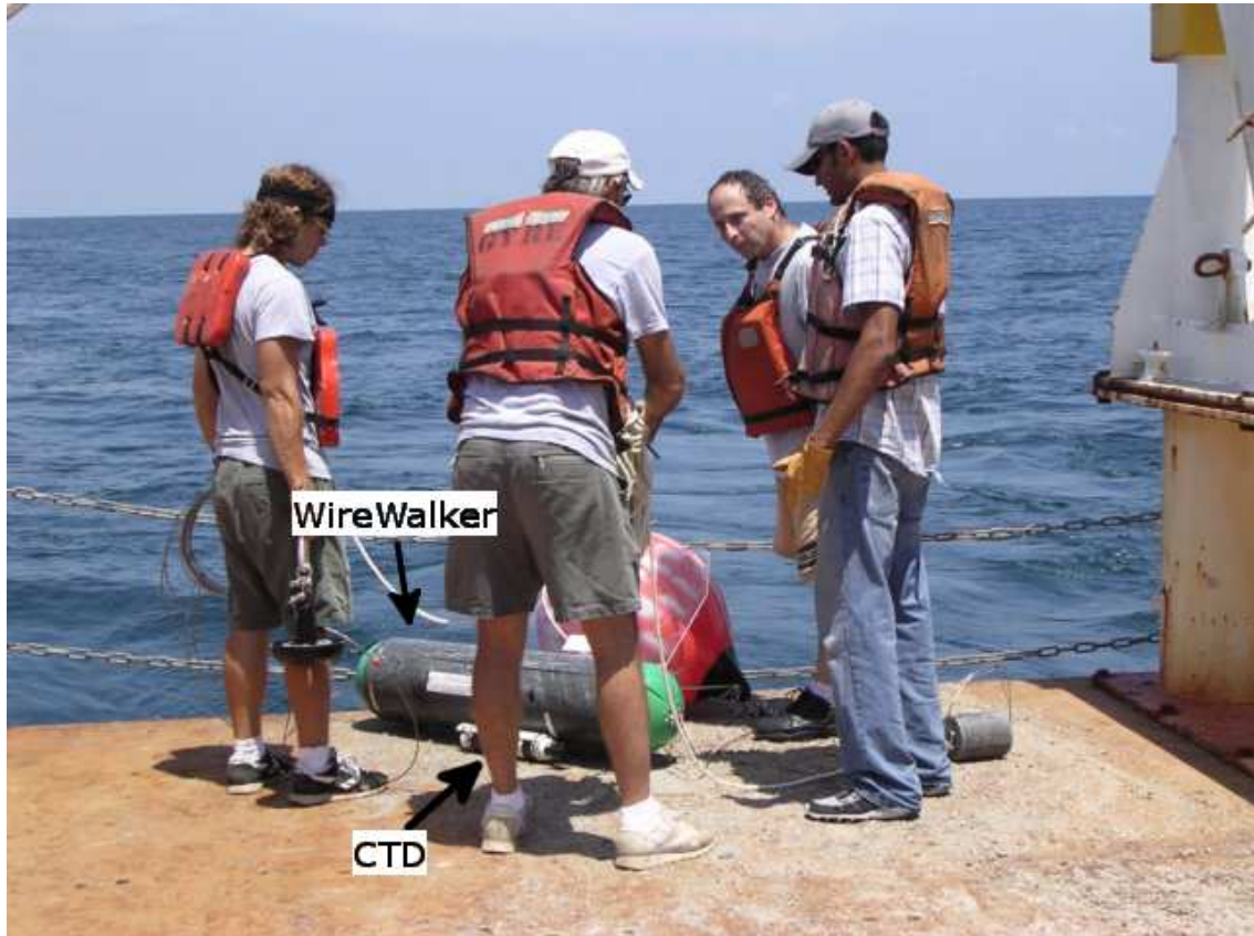
Figure 1.5: The CTD attached at the center of the WireWalker was ready to be lowered into the sea for autonomous profiling powered by surface wave energy (photograph courtesy Dr. Ayal Anis).
