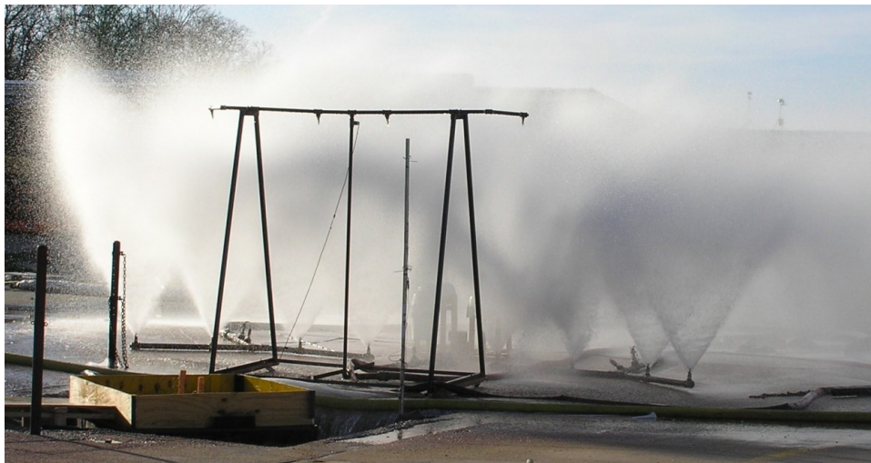
Fig. 70. Upward-oriented full conical water spray system
