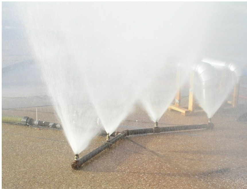
Fig. 29. Upward conical water sprays from March 2009 MKOPSC LNG experiment
