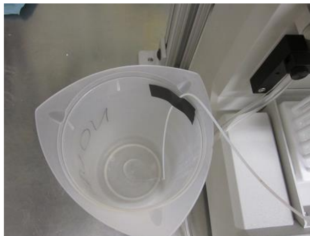
Figure 84: Fraction Collector Diverted Liquid
