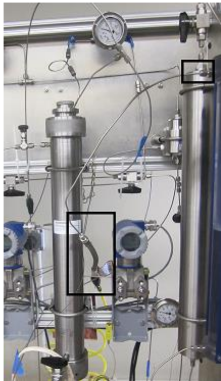
Figure 55: Air Connection for Refill Tank
