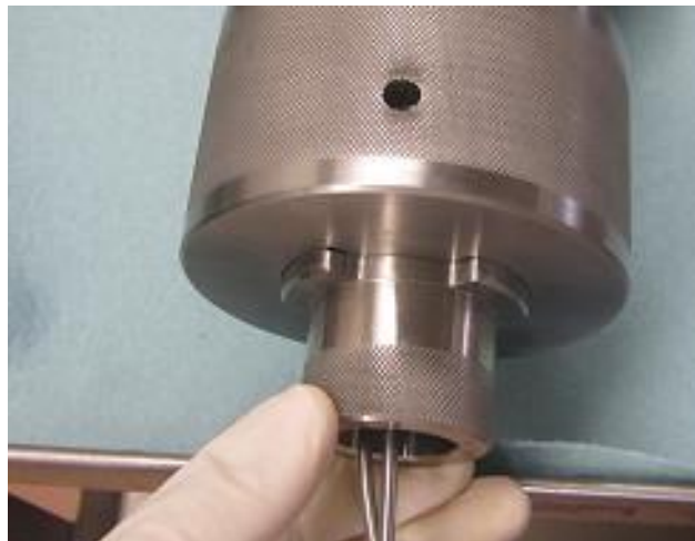
Figure 63: Bottom Plug Insert
