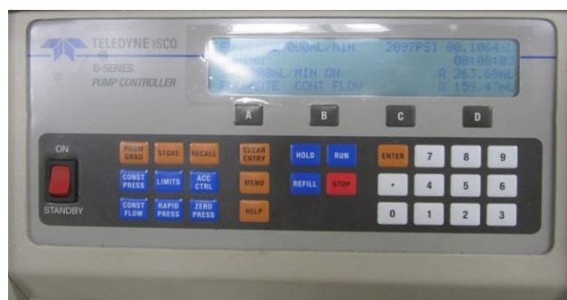
Figure 13: Pump Control Panel
