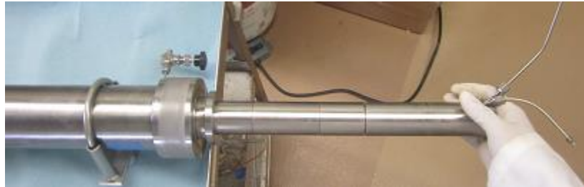
Figure 62: Spacer and Top Plug Inserted into Core Holder
