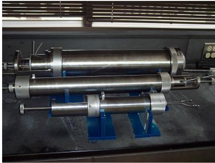
Figure 8: Small, Medium, and Large Core Holders
