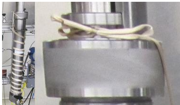
Figure 67: Heating Tape Attached
