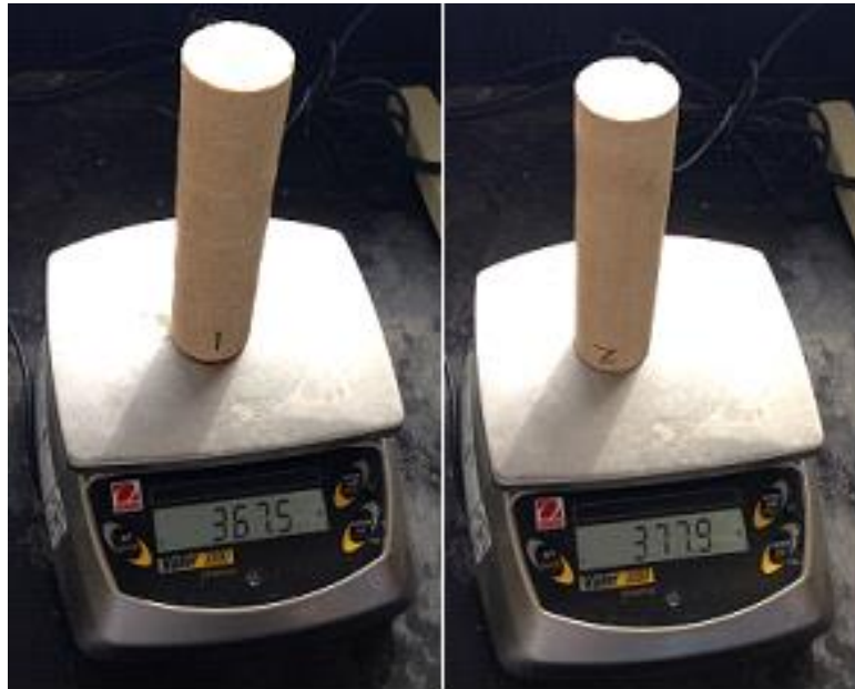
Figure 53: Saturated Core Weight
