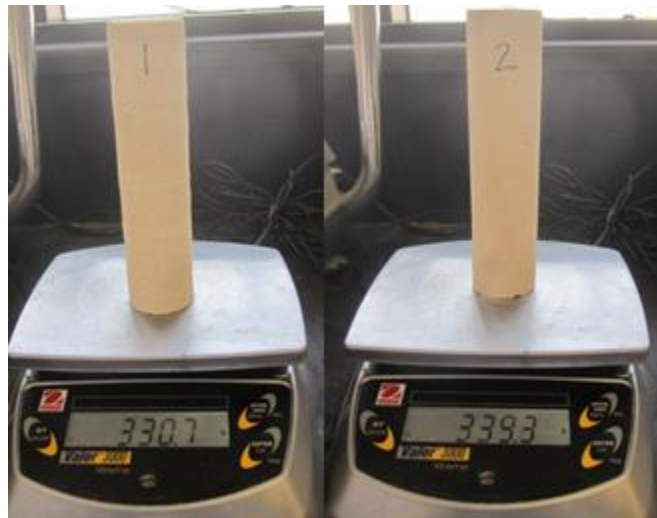
Figure 51: Dry Weight Measurement
