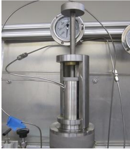
Figure 65: Secured Top Screw Cap
