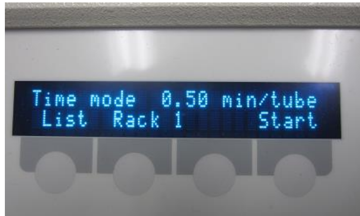
Figure 83: Fraction Collector Panel Setting
