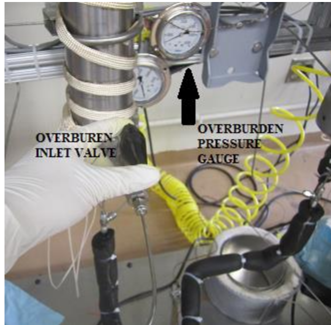
Figure 71: Overburden Pressure Gauge
