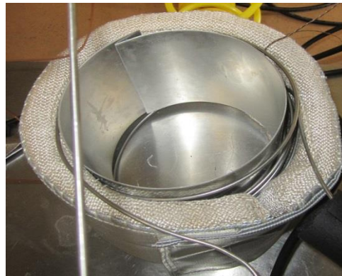
Figure 30: Fluid Heater with Hastelloy Tubing
