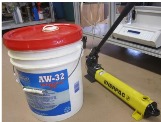
Figure 15: AW-32 Hydraulic Oil and Overburden Pump
