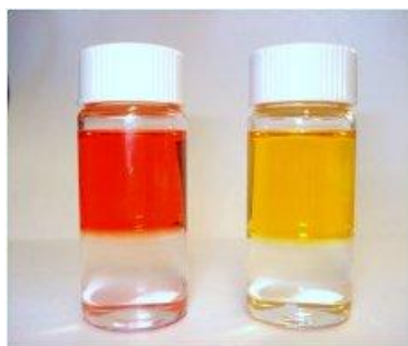
Figure 9. Phase selective solubility of the PIB-bound azodyes 52 (yellow) and 53 (red) in heptane (top phase) versus acetonitrile (bottom phase).
