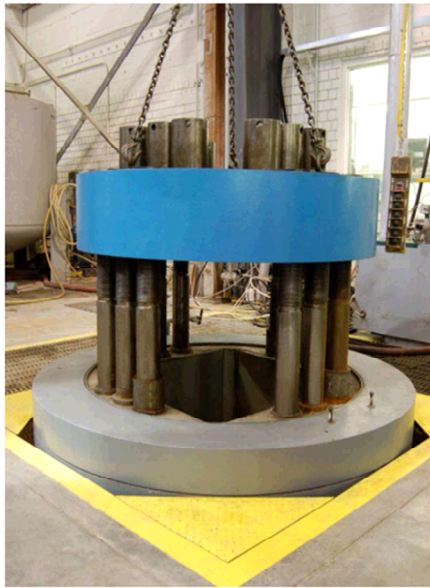
Figure 11.1 TerraTek's large multi-axial stress frame and Niobrara boulder acquired from the quarry in Colorado (Ghassemi and Suárez-Rivera 2012)
