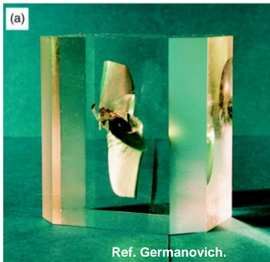
Figure 8.4 Crack growths of 3D wing-crack in uniaxial compression (Dyskin et al. 2003; Germanovich and Dyskin 2000)
