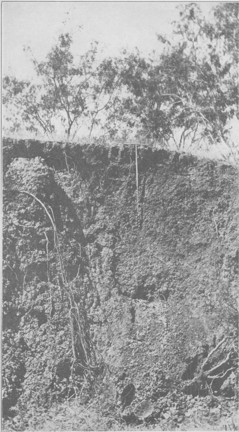
Figure 32. Soil profile of Crockett fine sandy loam. The topsoil is about eight inches deep and is underlain by dark crumbly clay.
