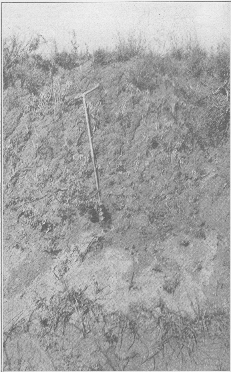
Figure 59. Soil profile of Miles find sandy loam (near Snyder) in the Rolling Plains Region. Note the layer of calcium carbonate which lies four feet beneath the surface.
