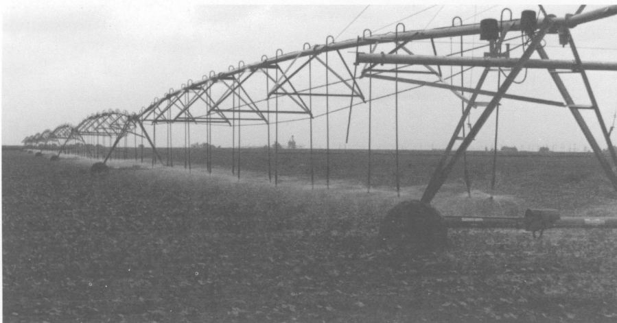
Figure 13. A sprinkler irrigation system equipped with drop hoses that deliver the water close to the soil surface, thus reducing evaporation.
