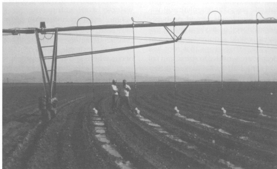
Figure 15. The LEPA (Low Energy Precision Application) irrigation system applies water to furrow-diked land at a low pressure, thus resulting in energy savings, precision water application, and reduced evaporation.
