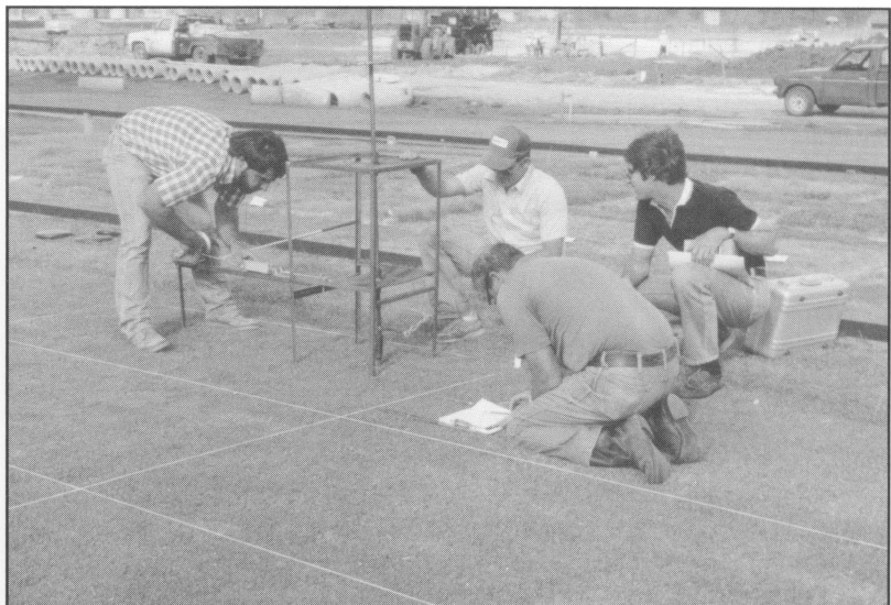
▲ Figure E-2. View of the compression displacement-turf tear-traction simulation apparatus.
