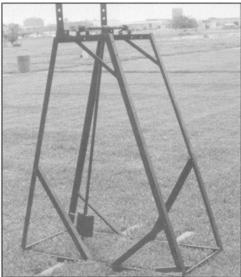
▲ Figure E-1. View of the divot simulation apparatus. A closeup of the resulting divot openings is shown in the color section, page 29.
