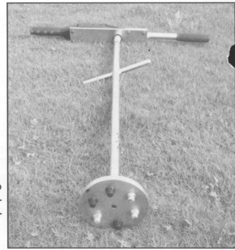
Figure E-3. Two views of the modified traction simulation device.
