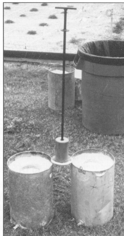
Figure G-1. View of the root zone compression apparatus (right) and the circular columned containers (below).
