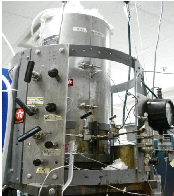
Figure 4.7. Steam generator used to prepare the injection fluid.
