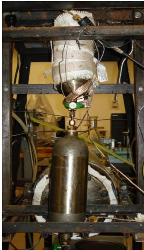
Figure 4.9. Two large separators were used to collect produced fluids.
