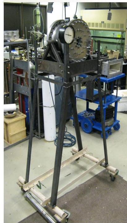
The Physical Model is Mounted on a tall Standing to Reduce the Length of Injection Line and Minimize Heat Losses
