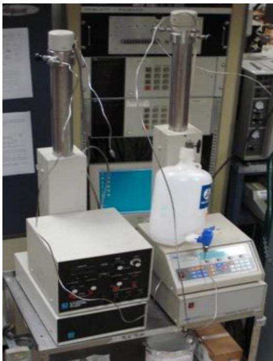
Figure 4.6. The positive displacement pumps used to inject solvent and water into the steam generator.
