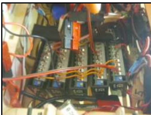
Fig. B.10. Secure dual mic phantom adapters inside fuselage via Velcro strap.
