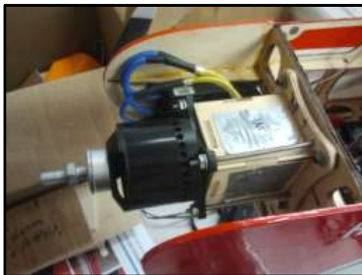
Fig. B.3. Motrolfly brushless motor mounted to UAV fuselage.
