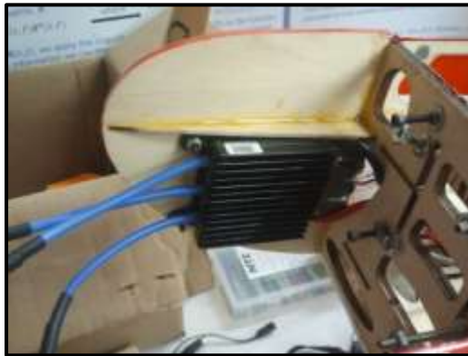
Fig. B.2. Hobbywing ESC mounted to UAV fuselage.
