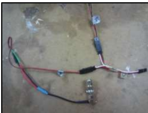
Fig. B.6. UAV microphone, Y-harness and BNC-to-Servo cable.
