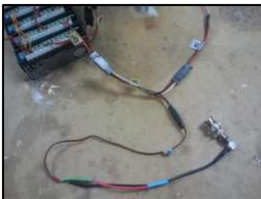
Fig. B.7. Dual mic phantom adaptor, UAV microphone, Y-harness and BNC-to-Servo cable.
