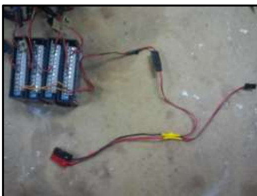
Fig. B.8. Dual mic phantom adaptor to Servo-to-Anderson Y-harness.
