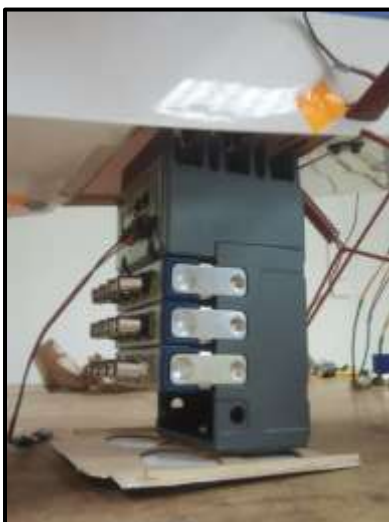
Fig. B.11. Insert cRIO DAQ into fuselage.
