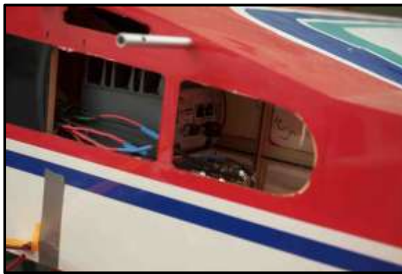
Fig. B.13. BNC cables connected to corresponding cRIO DAQ channels.
