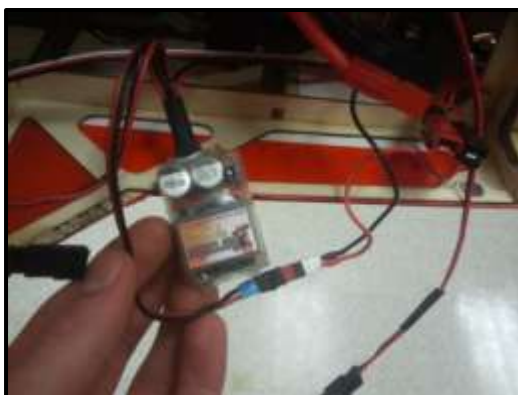
Fig. B.4. Hercules BEC connected to Hobbywing ESC.
