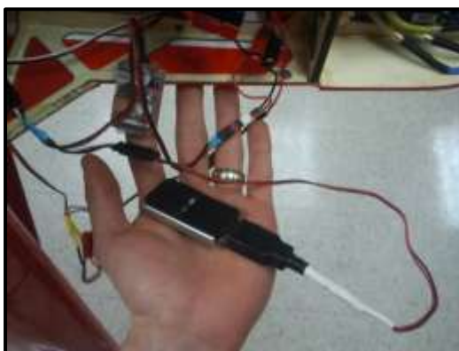
Fig. B.5. GPS data logger connected to BEC.
