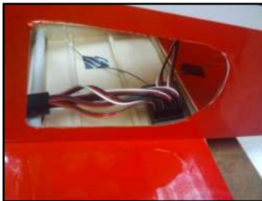
Fig. B.14. Futaba receiver connected to the control surfaces.
