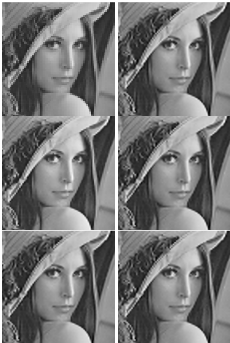
Figure 5.1: The Lenna test image. Down-sampled image (top left); global L^1 -reconstruction using the Interior Point method with \epsilon = 0.01 (top right); third Jacobi iteration of the domain decomposition algorithm using the Interior Point method with \epsilon = 0.01 (middle left); third Jacobi iteration of the domain decomposition algorithm using the Interior Point method with \epsilon = 0.05 (middle right); third Jacobi iteration of the domain decomposition algorithm using the Augmented Lagrangian method run for 10 steps (bottom left); third Jacobi iteration of the domain decomposition algorithm using the Augmented Lagrangian method run for 100 steps (bottom right).
