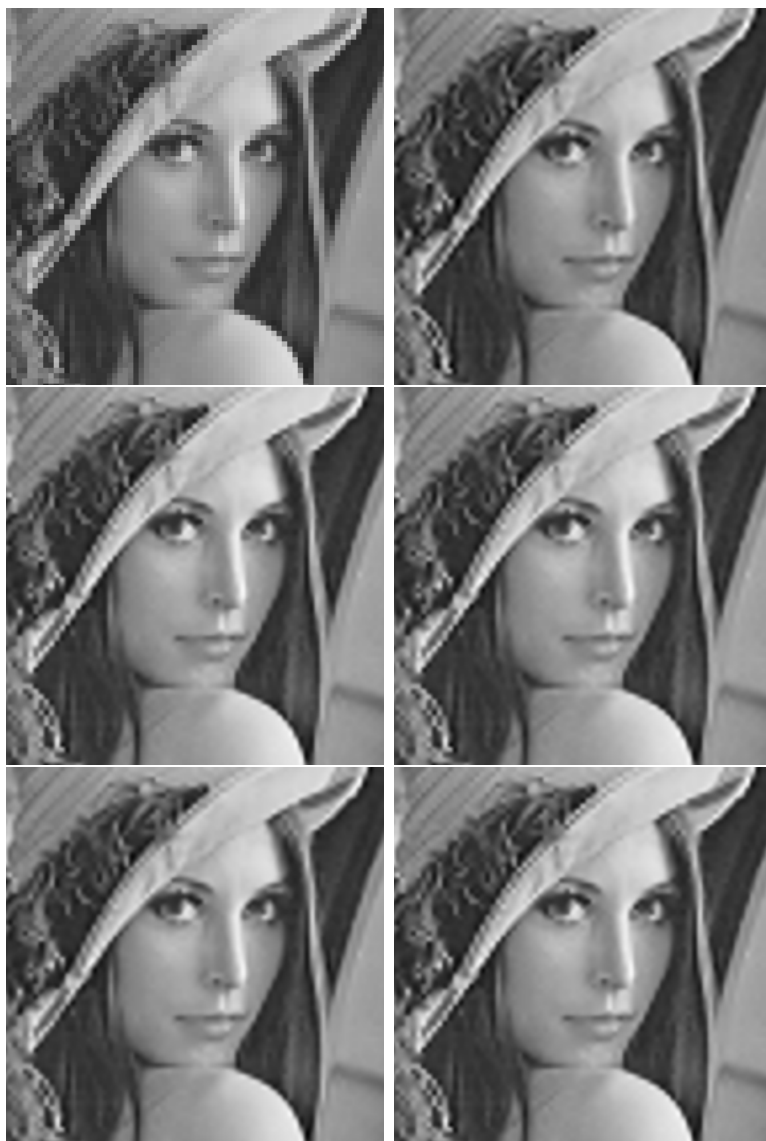
Figure 5.3: The Lenna test image. Down-sampled image (top left); global L^1 -reconstruction using the Interior Point method with \epsilon = 0.01 (top right); fourth iteration of the approximate local algorithm for a 1 \times 1 local domain with a one cell interpolatory ghost layer using an Augmented Lagrangian solver (middle left); tenth iteration of the approximate local algorithm for a 1 \times 1 local domain with a one cell interpolatory ghost layer using an Augmented Lagrangian solver (middle right); tenth iteration of the approximate local algorithm for a 1 \times 1 local domain with a one cell relaxed ghost layer using an Interior Point solver (bottom left); tenth iteration of the approximate local algorithm for a 1 \times 1 local domain with a two cells interpolatory ghost layer using an Interior Point solver (bottom right).
