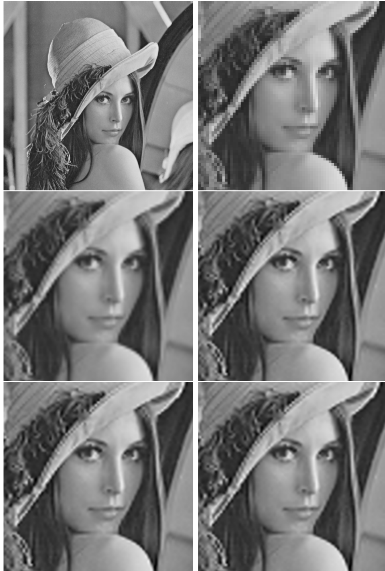
Figure 3.2: The Lenna test image. Original image (top left); down-sampled image (top right); standard bi-cubic reconstruction (middle left); global L^1 -reconstruction using the Interior Point method (middle right); global L^1 -reconstruction using 10 steps of the Augmented Lagrangian method (bottom left); and global L^1 -reconstruction using the Augmented Lagrangian method reached to the same functional the Interior Point method does (bottom right).
