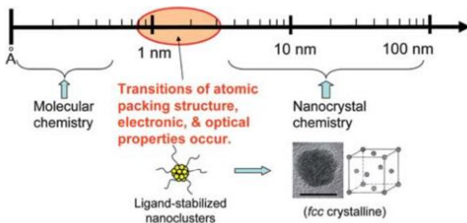
Fig. 9 Metal nanoclusters fill the gap between molecular chemistry and nanocrystals. The scale bar is 5 nm [59].
