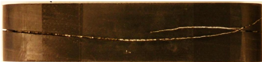
Fig. 15 – Well-cemented natural fracture
