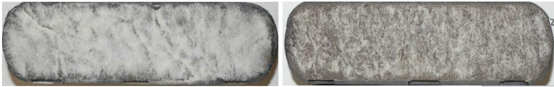
Fig. 8—Placement of 100-mesh sand on rough fracture surface at 0.10 lb/ft 2 (right) and 0.03 lb/ft 2 (left)
