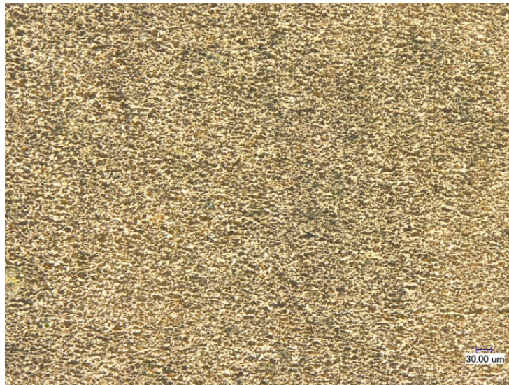
Figure 12. Optical microscopy images of the Fe-1.42Mn-1.56Si-0.32C samples after 950°C 1hr + ECAE 4E processing
