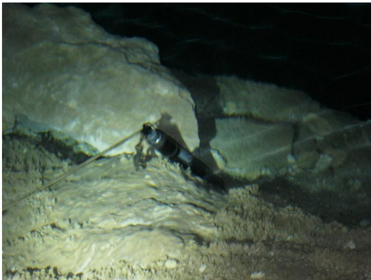
Fig. 3.2. Water Quality Monitor deployed at Church Cave.
