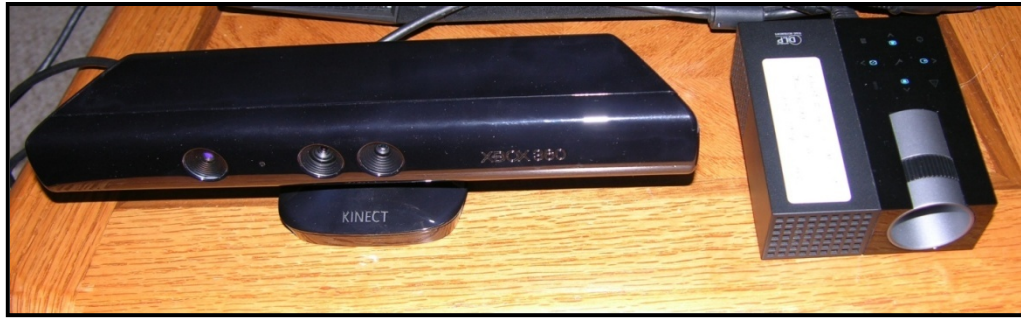
Figure 3. The proposed SAR system includes the Kinect sensor and a projector
