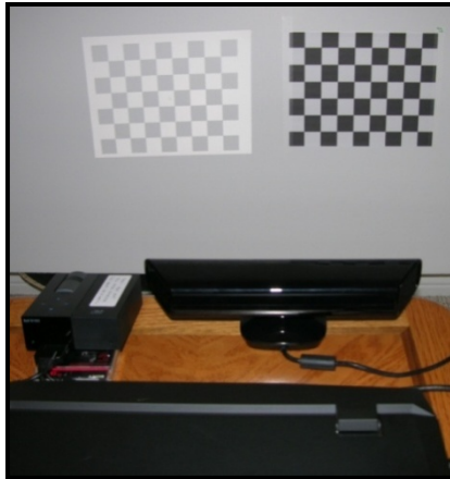
Figure 16. RGB camera acquisition of real and projected calibration targets
