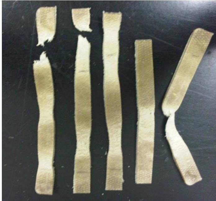
Figure 39. Shows the tensile tested specimen for 10% vol. MAHEMP
