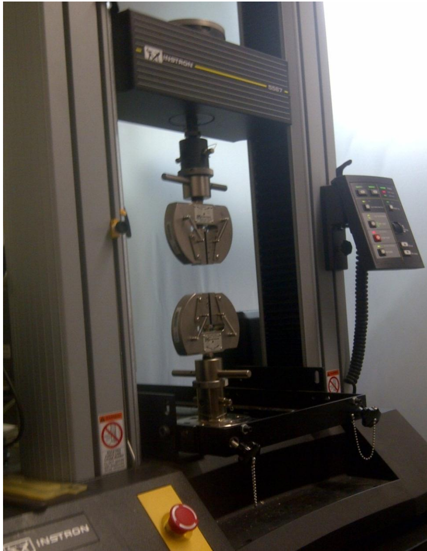
Figure 15 Tensile and flexural test performed on Instron 5567
