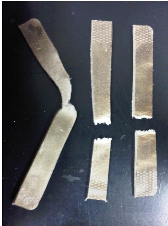
Figure 40 Failure of 10%, 20% and 30% vol. MAHEMP
