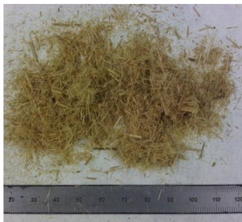
Figure 10. Grinded fiber using liquid nitrogen
