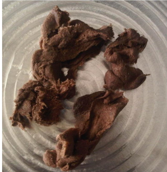
Figure 12 The lump of composite formed from one batch of melt mixing from the compounding machine.
