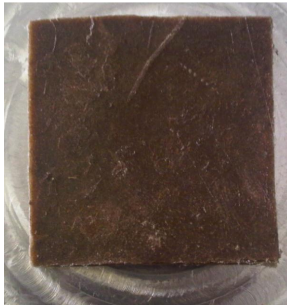
Figure 13 Plank of compressed composite from compression molding
