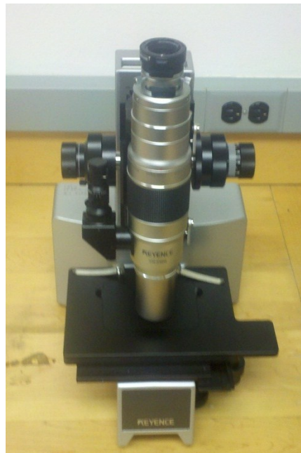
Figure 19. The figure displays the Keyence VH-Z500 lens attached to the lens holder.
