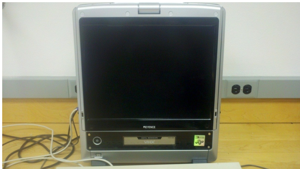
Figure 18. The figure displays the Keyence VHX-600 digital optical microscope.
