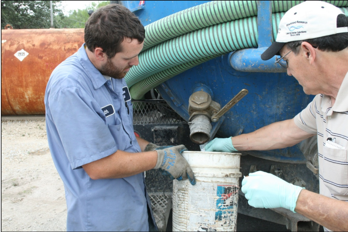
Collecting known source septic tank sample directly from pump truck
