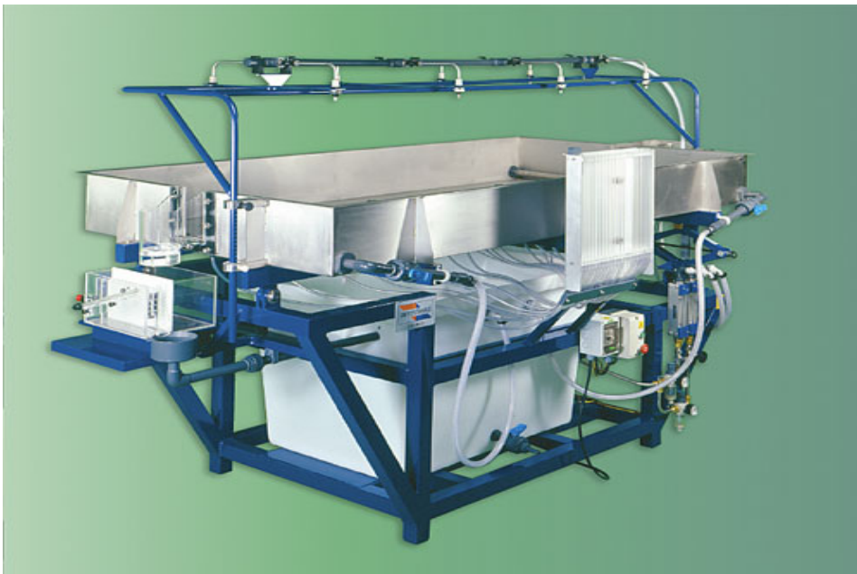
Fig.1 S-12 MKII-50 Advanced Hydrologic Systems (rainfall simulator).
