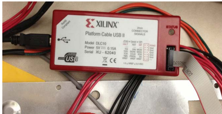
Figure 15: Xilinx downloader tool, on the left is the USB connection to the PC and on the right is the cable to the TMB.
