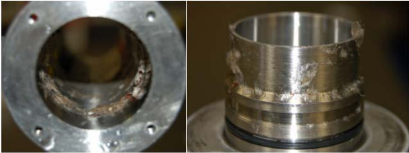
Figure 4.8. 1250 L/min cyclone inner wall, 6 minutes after adding 170 mg of the second-cut cotton linters.
