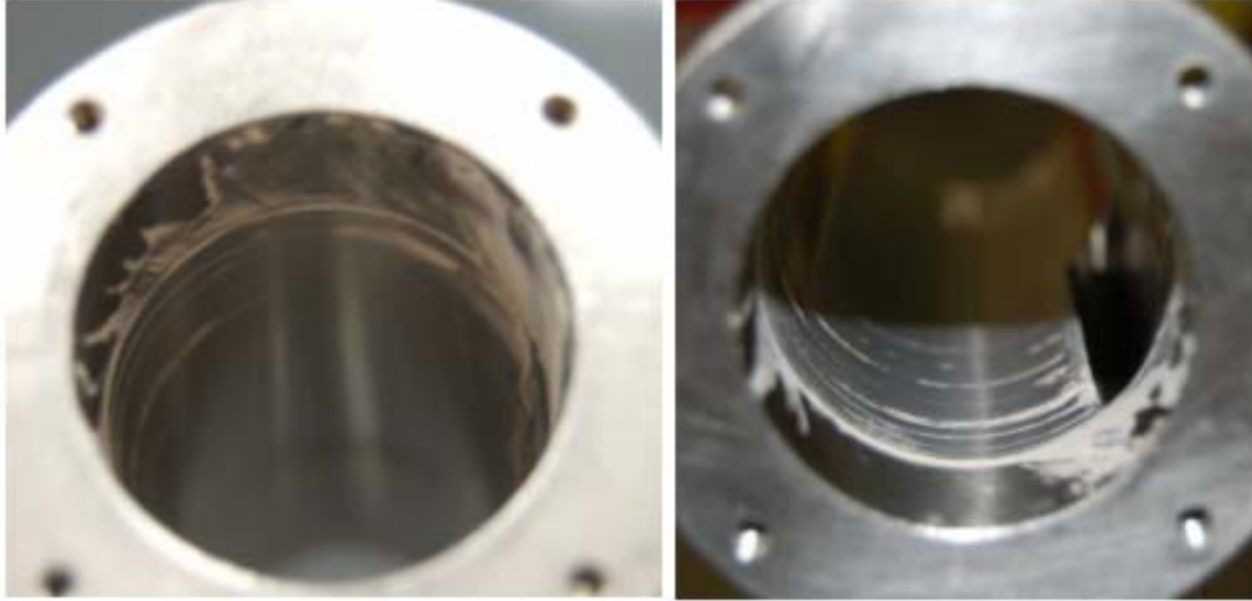
Figure 4.6. 1250 L/min cyclone inner wall, 6 minutes after adding 2000 mg of Arizona dust.
