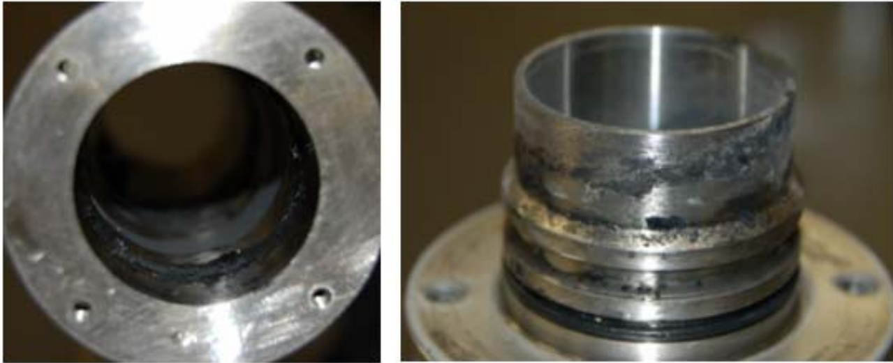
Figure 4.7. 1250 L/min cyclone inner wall, 8 minutes after adding 600 mg of ASHRAE test dust.
