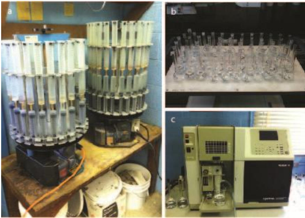
Fig. 3.6. Cation exchange determination for clays (b) and -40 screenings (a and c)
