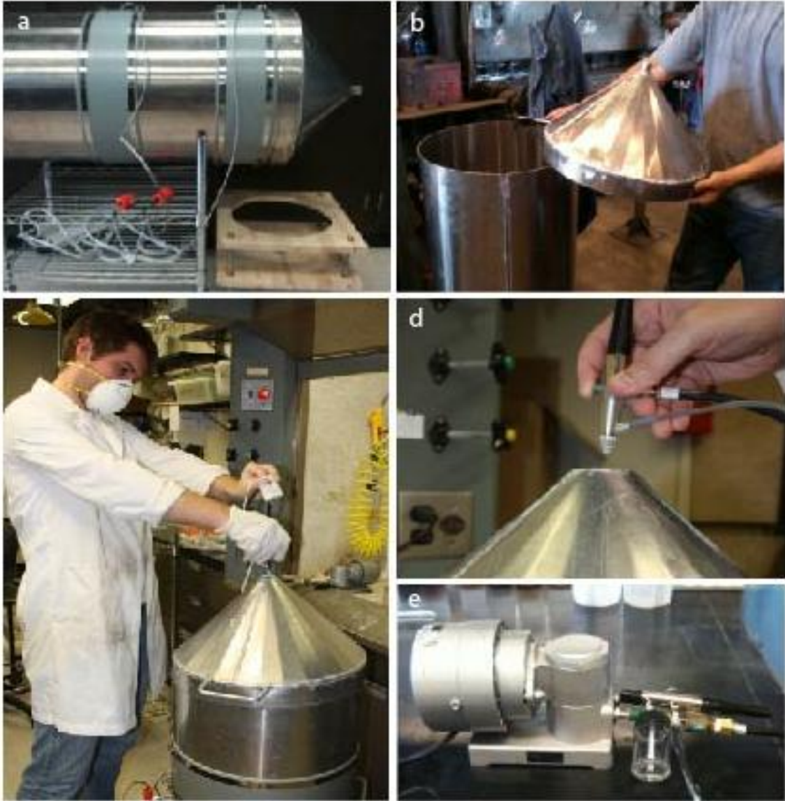
Fig. 3.5. Spray-drying procedure for reducing orientation effects during powder diffraction
