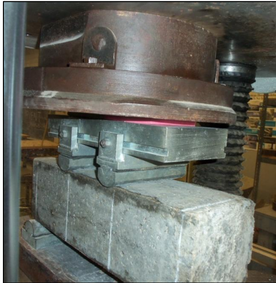
Figure 4.8. Concrete beam in three-point flexural strength testing apparatus.
