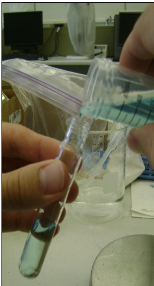
Figure 3.9. Transfer of diluted test solution to glass test tube.
