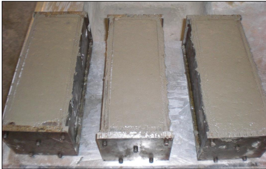
Figure 4.3. Drying shrinkage specimens.
