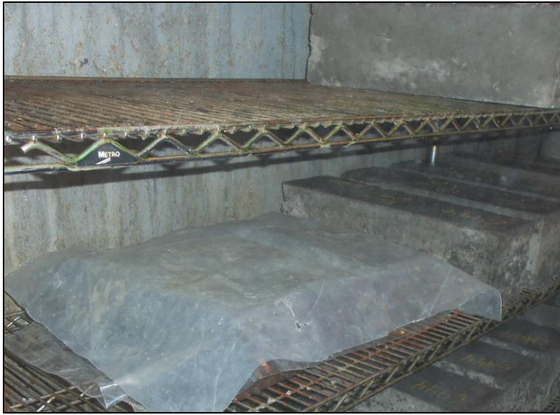
Figure 4.4. Concrete specimens curing in 100% moisture room.
