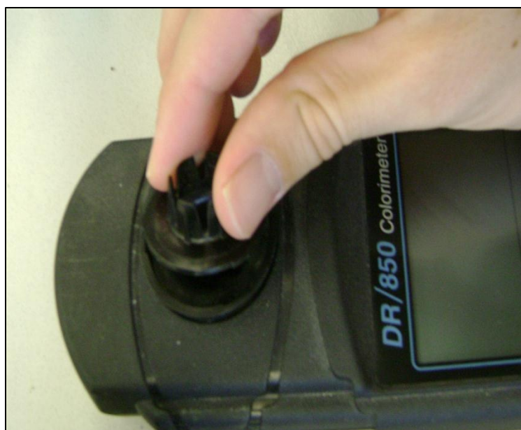
Figure 3.10. Installation of the 16-mm test tube adapter on the colorimeter.
