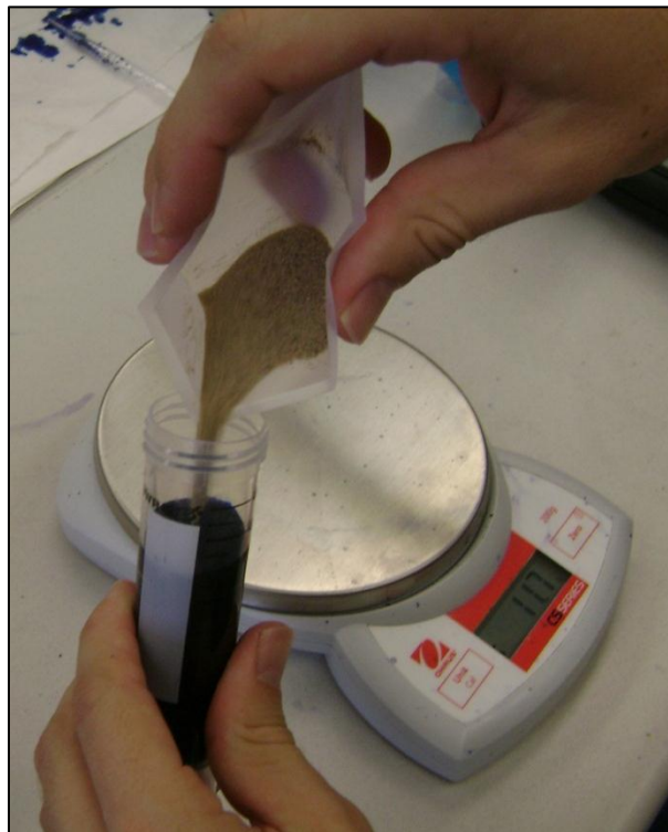
Figure 3.3. Combination of aggregate fines and methylene blue.
