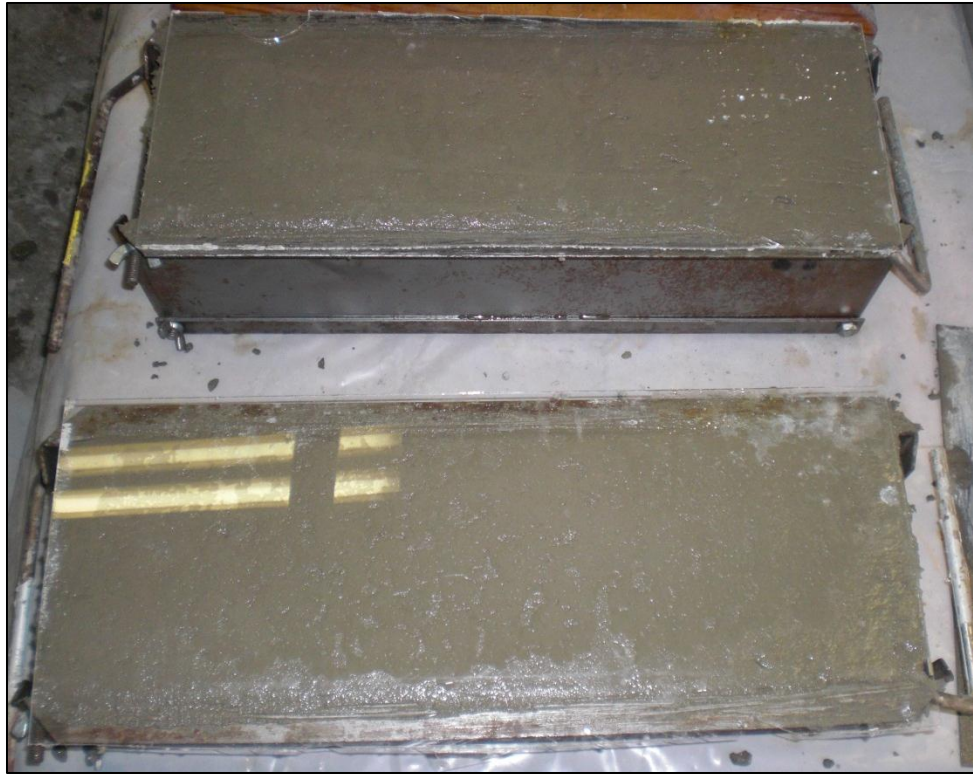
Figure 4.7. Flexural strength specimens.
