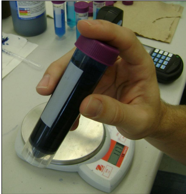
Figure 3.4. Shaking of test sample and methylene blue.
