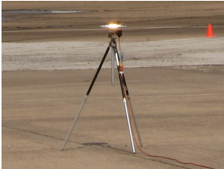
Figure 3.4: Target Beacon in Operation
