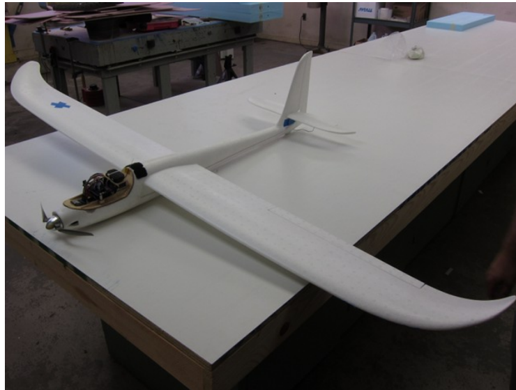
Figure 4.1: Multiplex Easy Glider Pro with Experimental Test Hardware Integrated
