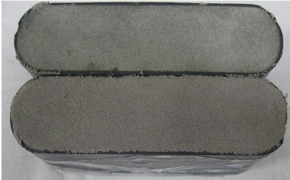
Fig 3.5 Experiment with Uniform Proppant Distribution
