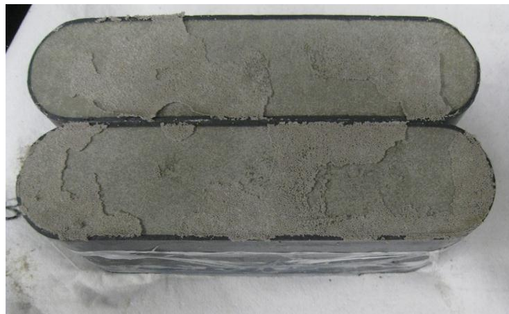
Fig 3.2: Dried and Crushed Proppant at High Closure Stresses
