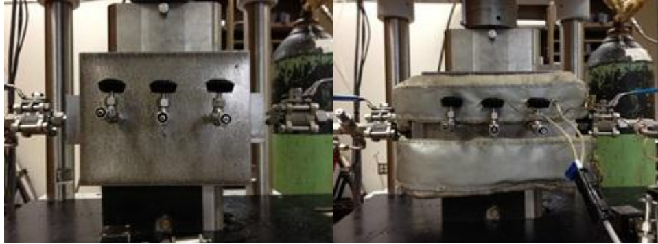
Fig 2.12: Final Assembly of the Conductivity Cell
