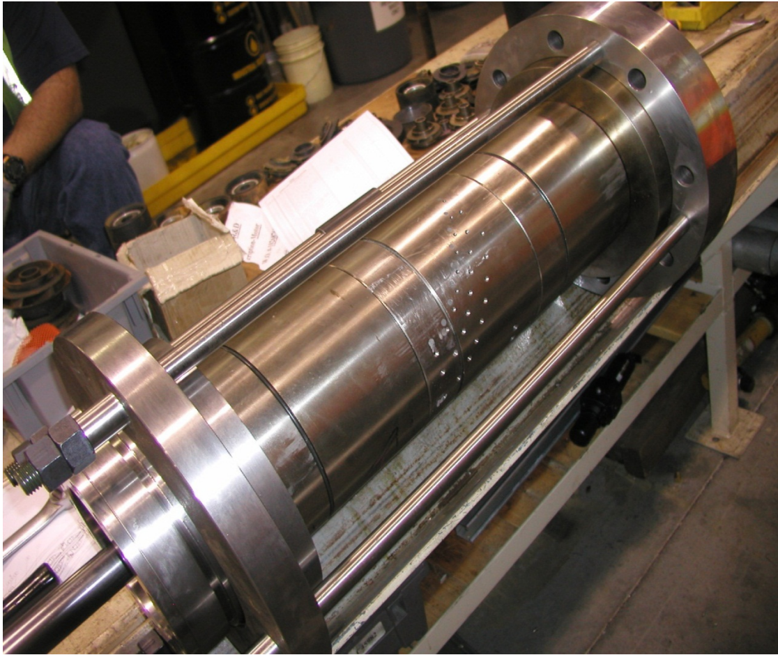
Figure 2.2 Pump with pressure taps
