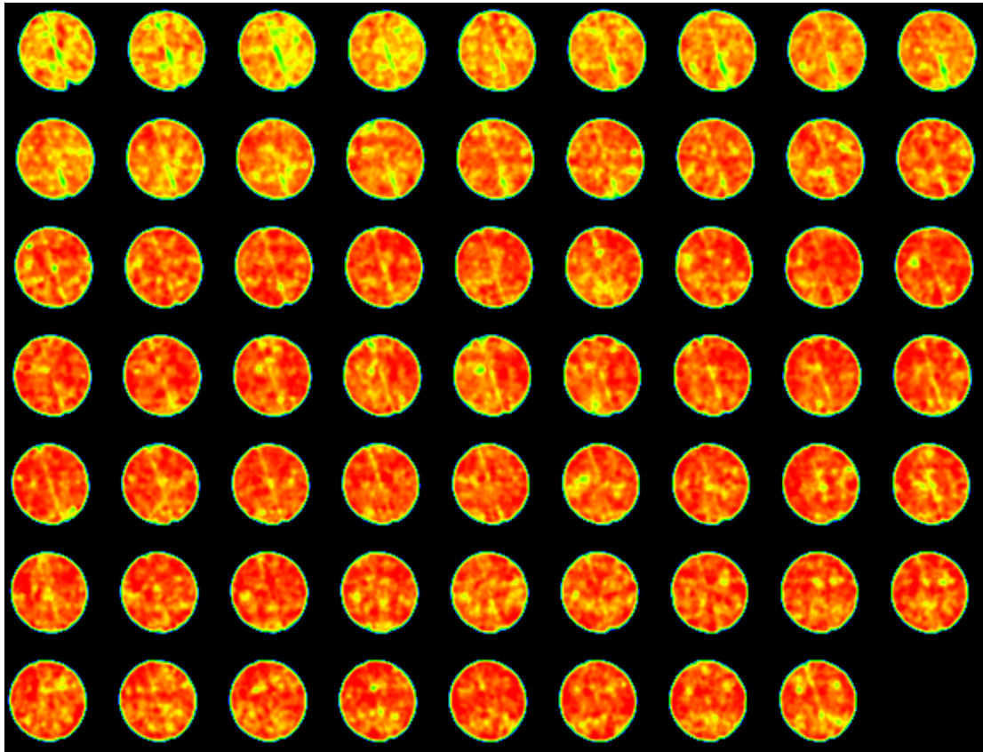
Fig.4.69 – Vertical Slice CT Images of Oil Saturated Core Flooded With 2 nd PV of VW (Exp#7)
