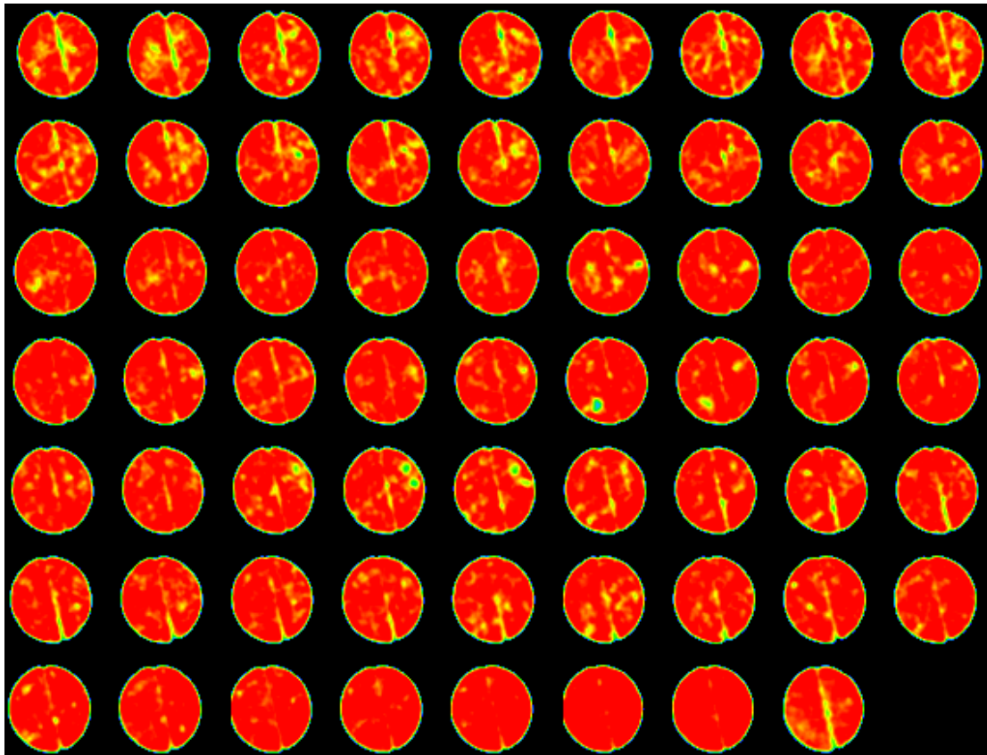
Fig.4.28 – Vertical Slice CT Images of Oil Saturated Core after Gel Treatment (Exp#4)
