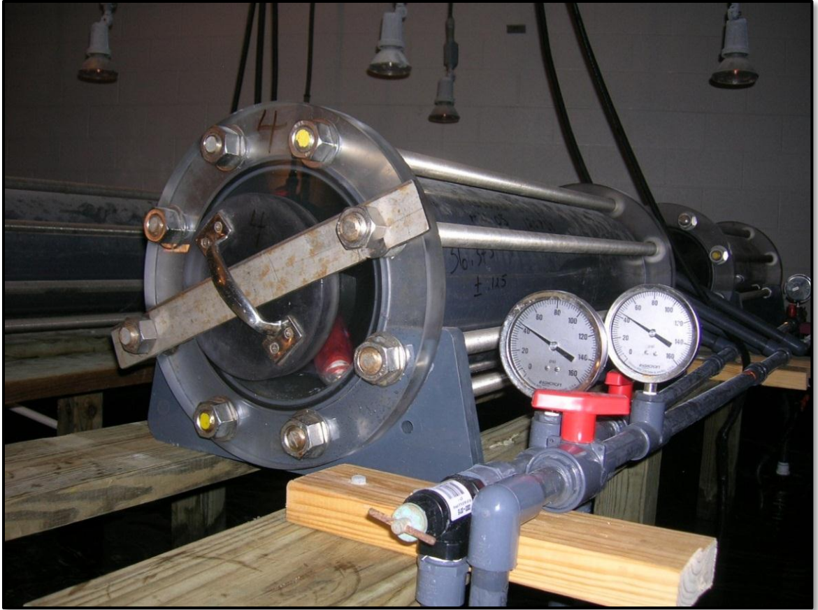
FIGURE 2. Photograph of a hyperbaric chamber used to simulate the pressure changes experienced by red snapper during hook-and-line capture events.
