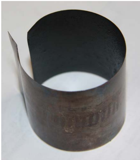
Fig. A.3 Top foil before assembly in a MMFB. The inner surface of the top foil coated with \text{MoS}_2
