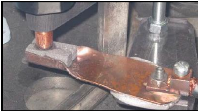
Figure 2-13: The INL fuel atomizer brush system [4].
