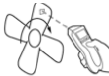
Figure 5-2: Illustration of how a non-contact tachometer works [23].
