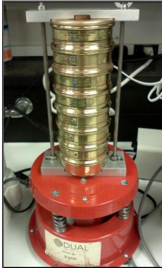
Figure 4-2: The Dual Manufacturing sieve used to filter the copper microspheres.
