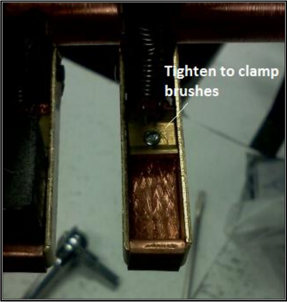
Figure 3-5: How a brush is attached and secured to the holder.
