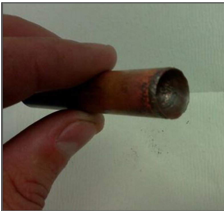
Figure 4-1: The concave cavity formed during atomization of the Cu pin.
