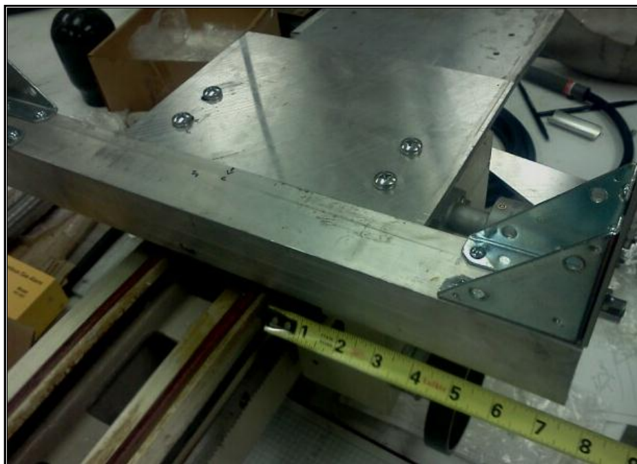
Figure 3-20: The catch pan column supports attached to the carriage cross beam.
