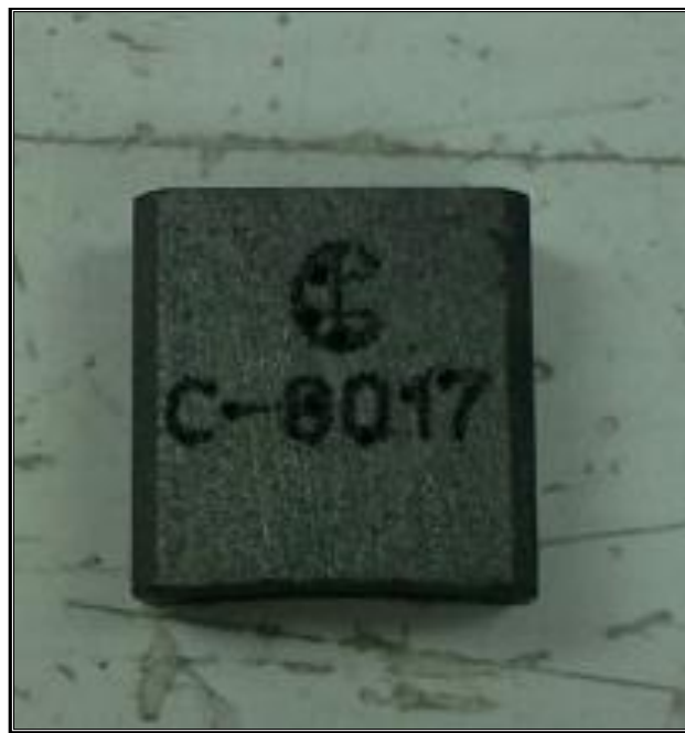
Figure 3-3: A single LFC554 electrographitic brush fabricated by Mersen.
