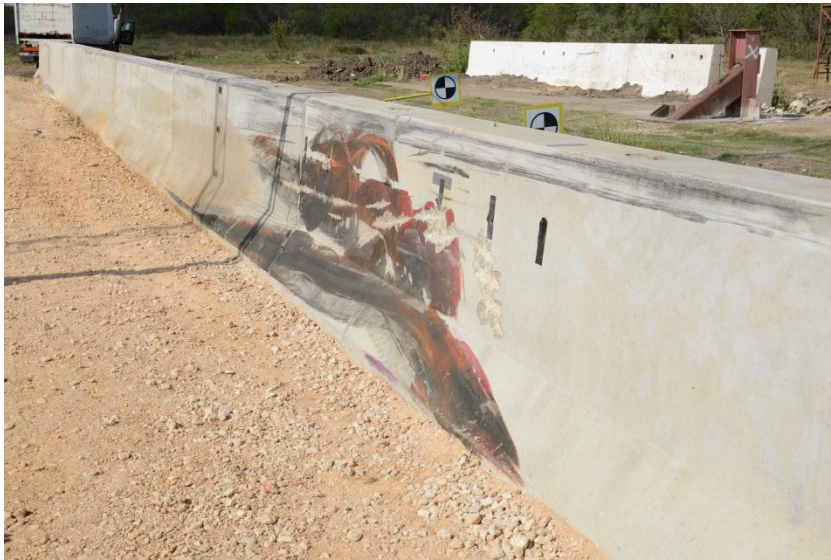
a) N.J shape barrier after test
