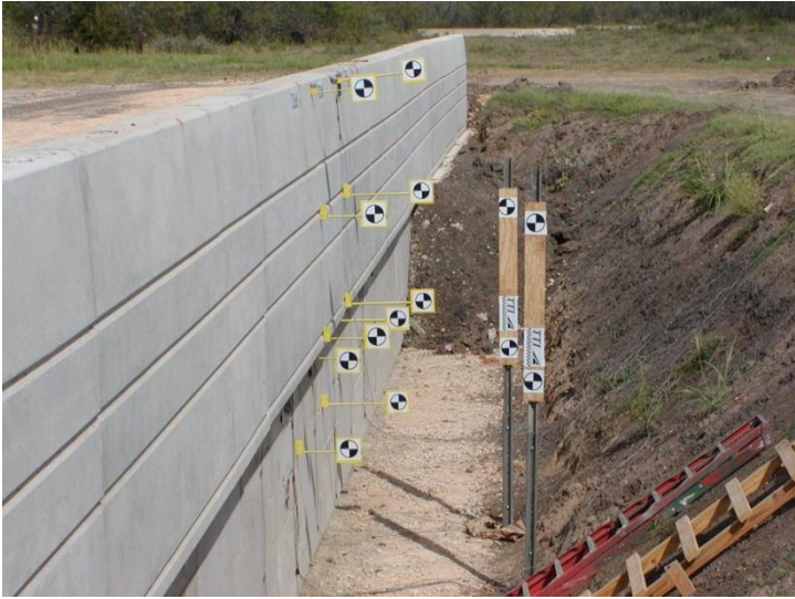
a) Targets to measure dynamic displacements
