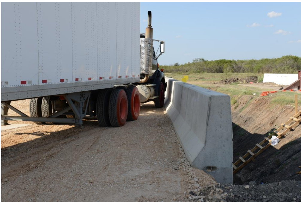
b) Set-up of the TL-5 full-scale showing the impact position
