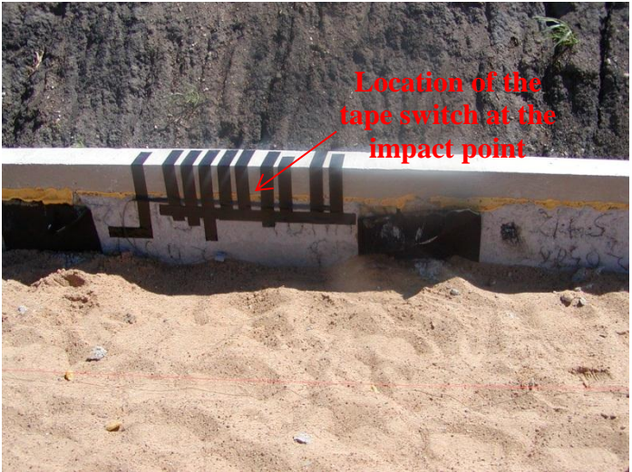
Figure D.12 Tape switch located at the impact point
