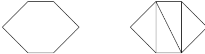
Figure I.1: Hexagonal cell versus triangle cells
