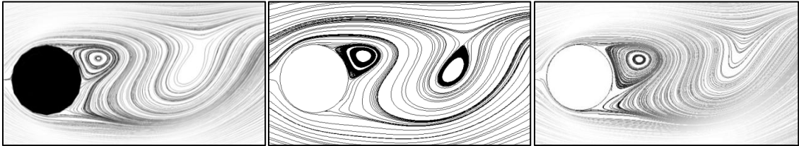
Figure 40. Streamlines for unsteady flow past a circular cylinder at Re = 100 . Left: IFEM vm, dg = 1 ; center: IFVM; right: STAR-CCM+.
