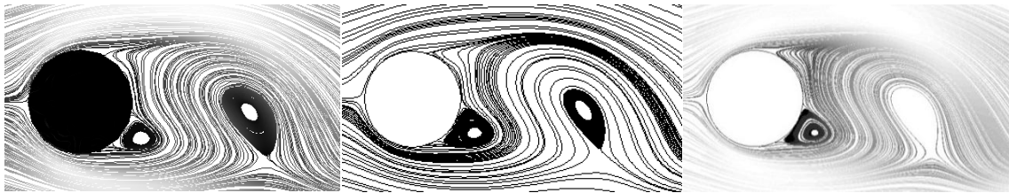
Figure 48. Streamlines for unsteady flow past a circular cylinder at Re = 150 . Left: IFEM vm, dg = 1 ; center: IFVM; right: STAR-CCM+.
