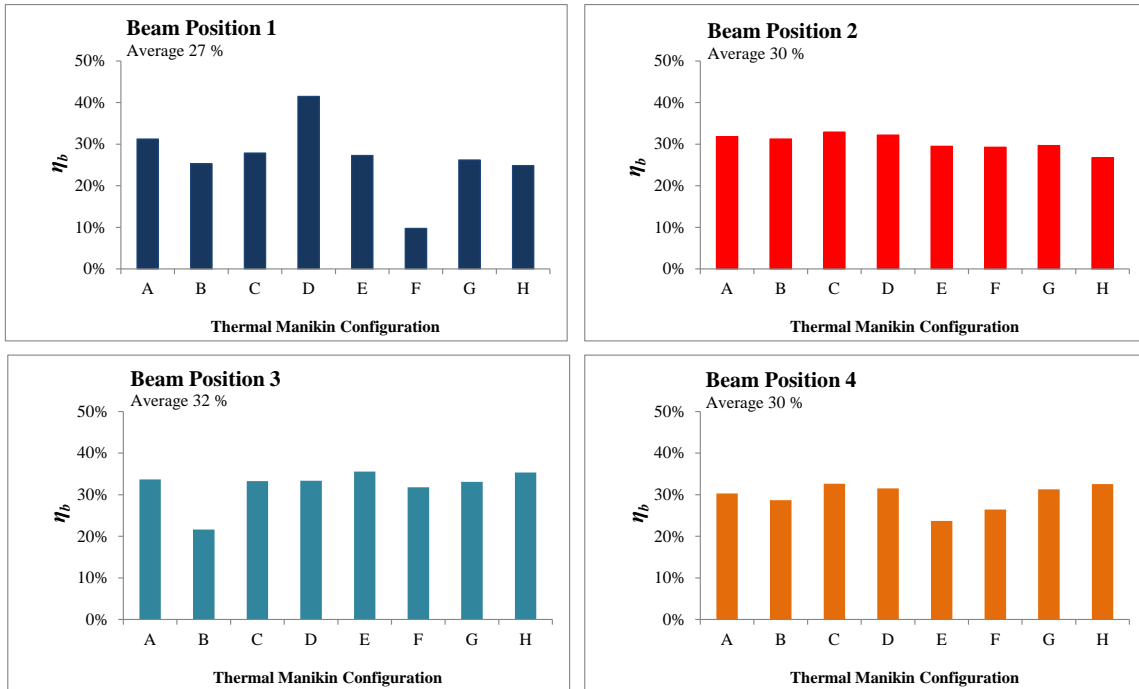
Figure 78. Beam efficiencies for the different configurations of thermal manikins grouped by the beam position.
