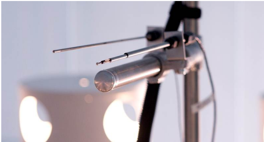
Figure 7. RTD probe and TSI omni-directional velocity probe pictured left to right, respectively.
