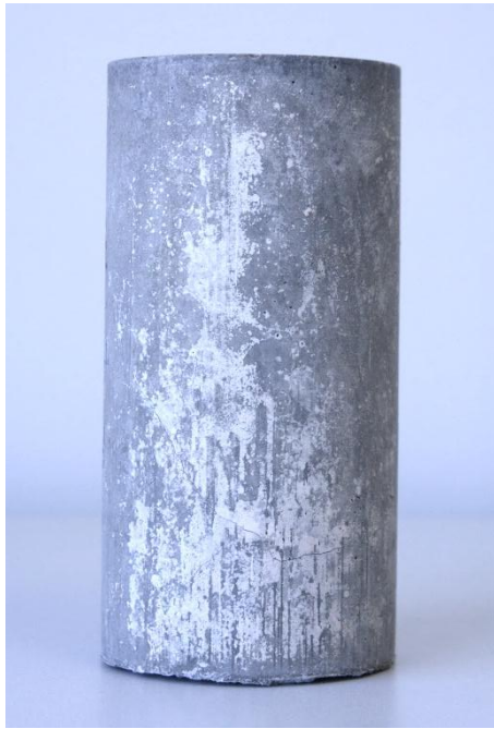
(a) Concrete Cylinder in Curing Room (with Hairline Cracking)
