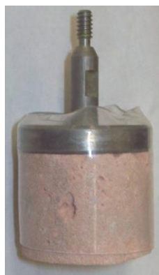
Fig. 2.2: A sample attached to the sample holder using the heat-shrinkable Teflon tubing.
