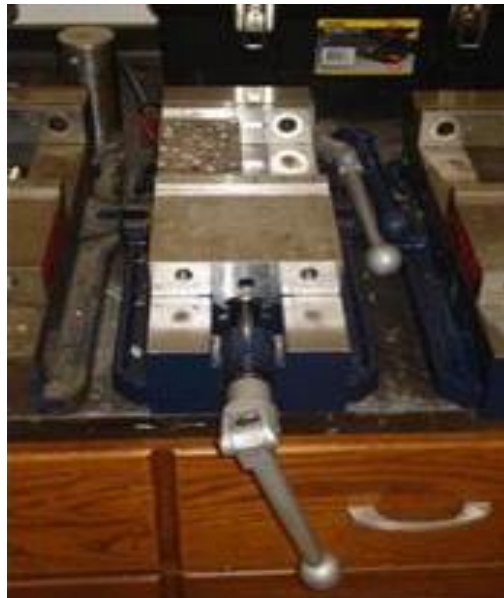
FIGURE 7 Magnetic gluing vice for field samples.
