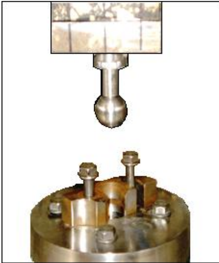
FIGURE 4 Three inch wide sample attached to ball and socket joint shown with movable base plate.
