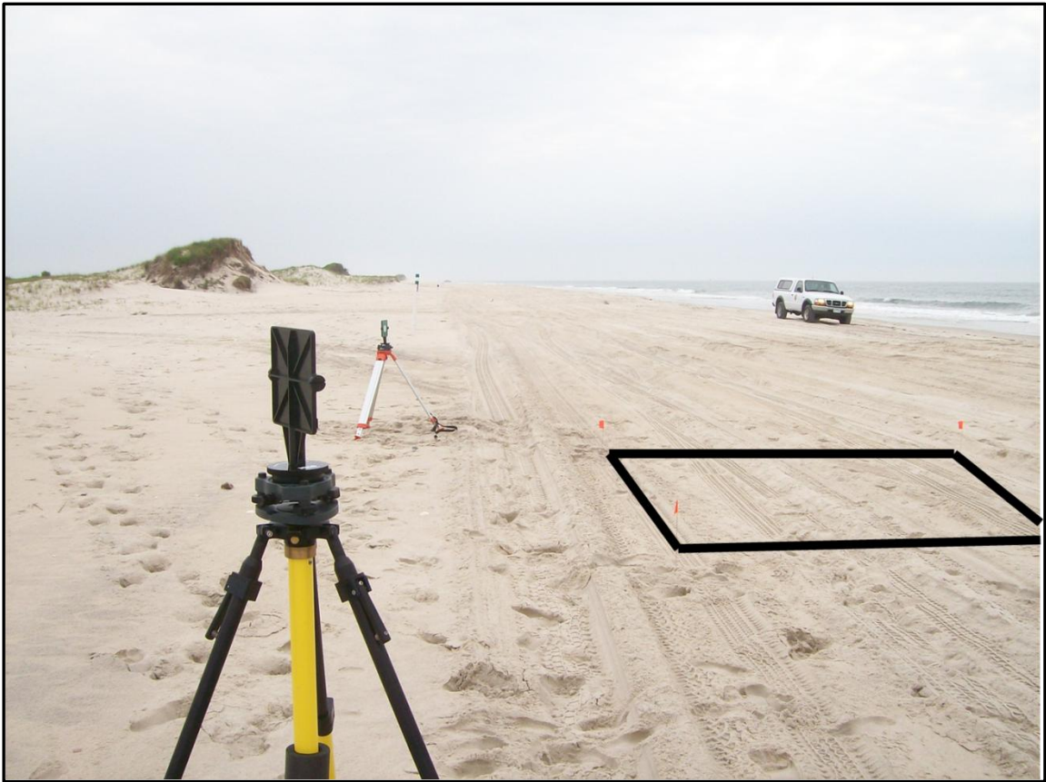
Figure 10. Location of targets in relation to the test plot and the Trimble GX 3D Scanner (The lines represent the test plot).
