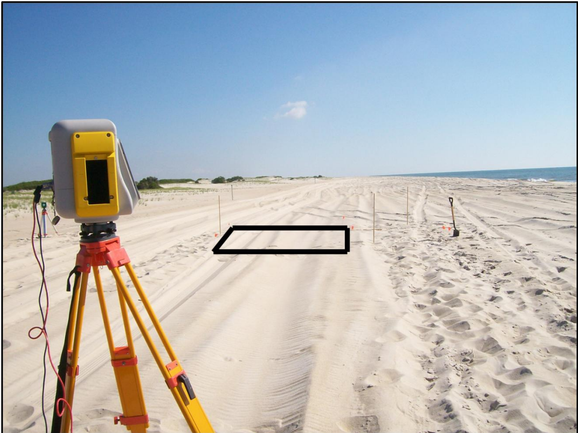
Figure 9. A typical placement of the Trimble GX 3D Scanner in relation to the test plot.
